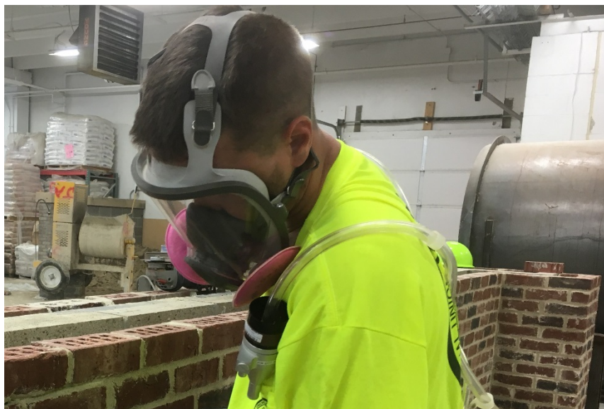
Figure 5 – Cyclone sampler in the breathing zone (NIOSH photo)
