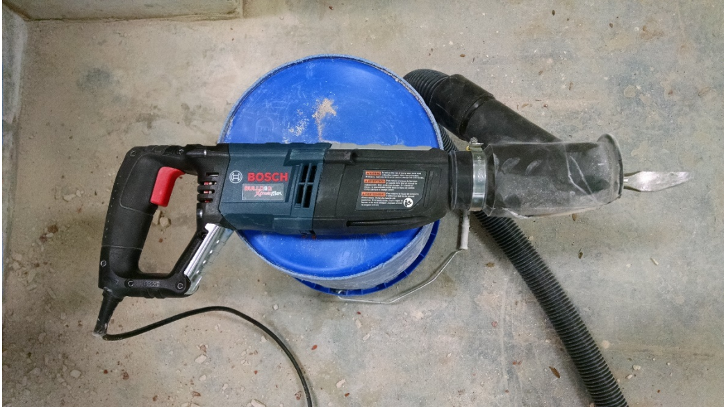
Figure 2 - Hammer drill with shroud and bit (NIOSH photo)
