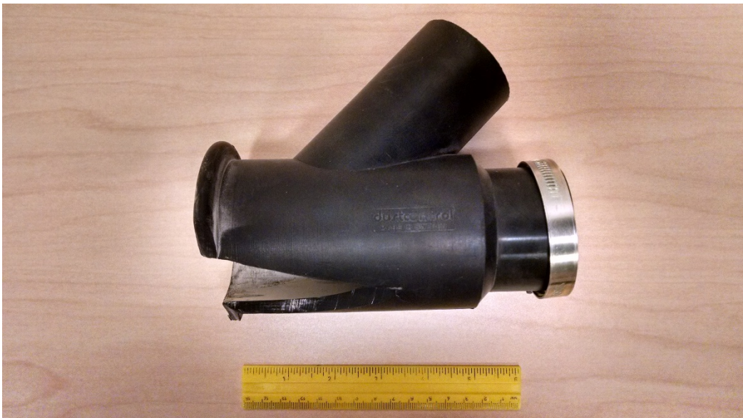
Figure 3 - On tool exhaust hood (NIOSH photo)
