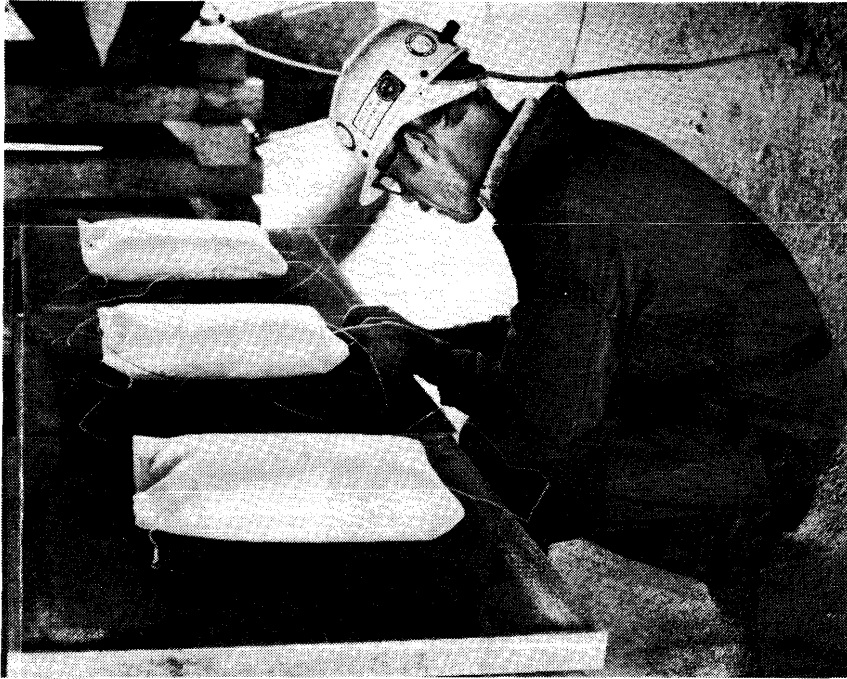
FIGURE 14. - Evaluating a commercial version of the Bureau-developed sheathed rock-breaker explosive charge.
