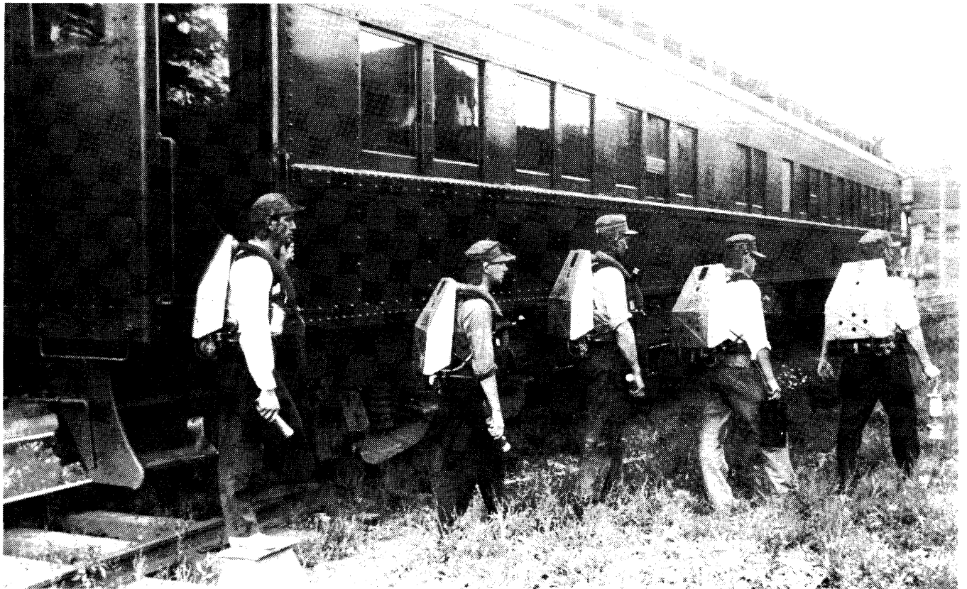
FIGURE 3. - Bureau of Mines mine safety railroad cars, which were equipped as movable safety and rescue stations.
