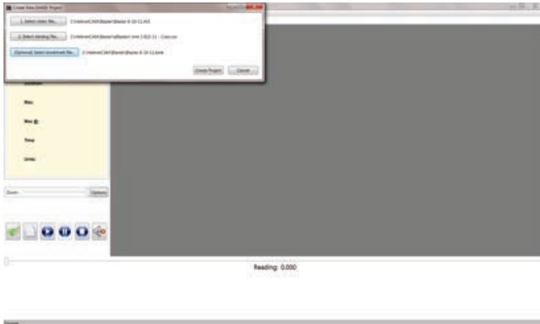
Figure 28. The Create New EVADE Project dialog box after all data file selections have been completed.
