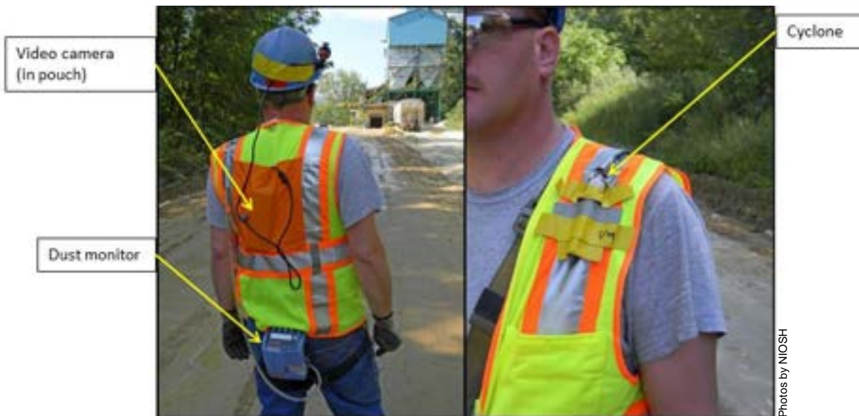
Figure 3. Setup of sampling devices for personal sampling.
