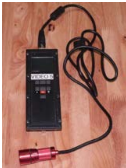
Figure 2. The V.I.O. Point-of-View video camera used in the Helmet-CAM, showing the body of the camera and the lens component (below the body) attached by cable.
