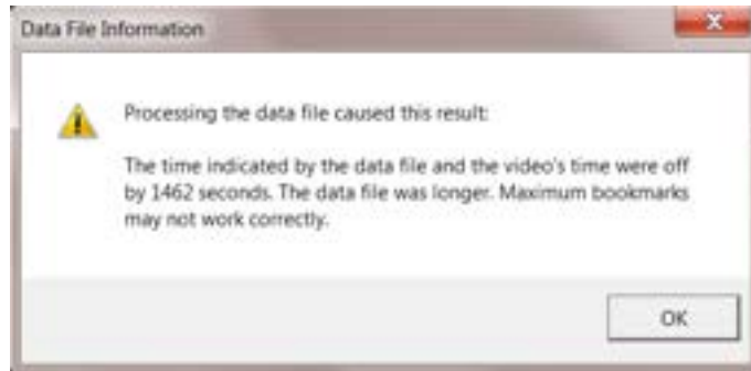
Figure 21. Data file information alert for time differential between video and dust concentration files.
