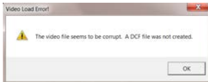
Figure 22. A Video Load Error! dialog box that appears during the Open command if the video file is corrupt.
