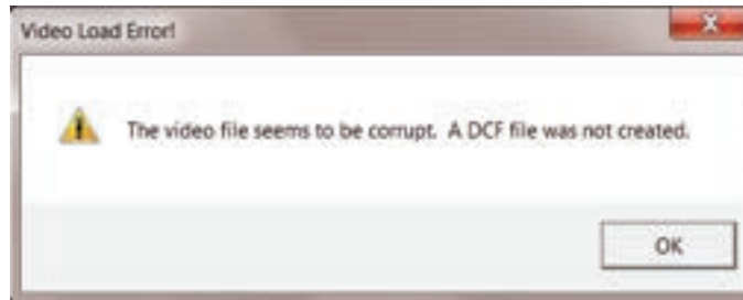
Figure 30. A Video Load Error! dialog box that appears during the New Project command if the video file is corrupt.
