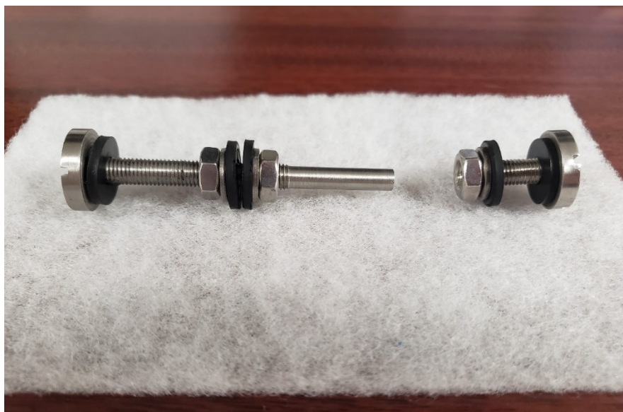
Figure 11: Sample Probe View Set Up as – Double (left) and Single (right)
