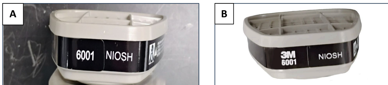
Figure 4: Example of fraudulent 6001 chemical cartridge (A) with similar cartridge label as genuine 3M 6001 (B), except for 3M missing on fraudulent chemical cartridges.
