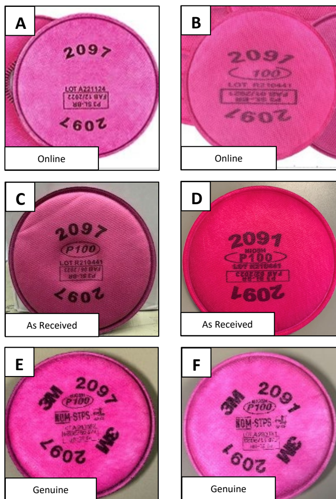
Figure 2: Examples of the appearance of fraudulent filters on the online marketplace (A and B), the appearance of these fraudulent filters when NIOSH received them (C and D), and the appearance of genuine 3M 2097 and 2091 P100 filters (E and F).
