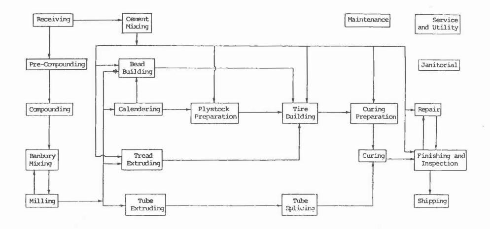
Figure 1. Production Stages in the Manufacture of Tires and Tubes.
