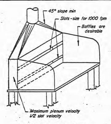
Q = 350 cfm/lineal ft of hood Hood length = required working space Bench width = 24" maximum Duct velocity = 1000 - 3000 fpm Entry loss=1.78 slot VP +0.25 duct VP
