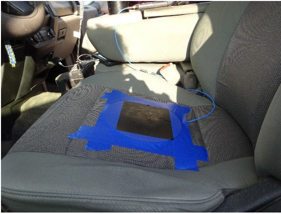
Figure B1. Rubber seat pad with embedded triaxial sensor for measuring WBV on the range operator truck seat. Photo by NIOSH.
