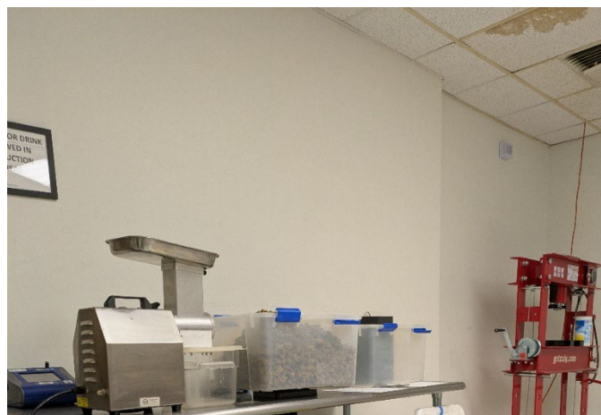
Figure A1. Grinding station showing the shredder and dried cannabis material. A DustTrak™, shown in the background on the left side of the work table, measured particulates generated during work tasks. Photo by NIOSH.
