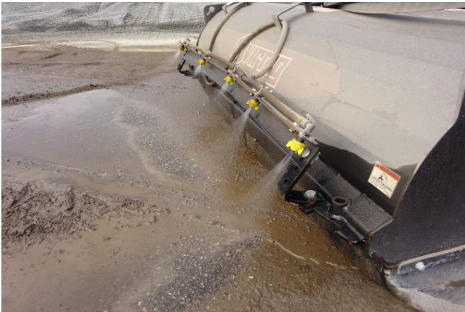
Figure A10. Water-based dust suppression nozzles attached to the rotary broom on the front of a skid-steer machine. Photo by NIOSH.
