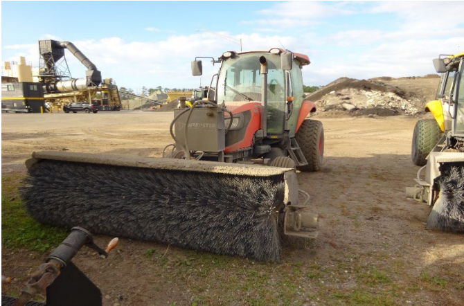
Figure A8. Rotary broom attached to a tractor used to sweep yard. Photo by NIOSH.
