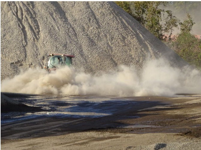
Figure A9. Tractor with front mounted rotary broom sweeping yard space. Rotary broom does not have a water-based dust suppression attachment. Photo by NIOSH.
