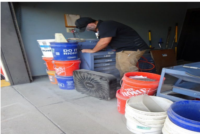
Figure A4. Laboratory QA/QC technician using compressed air to clean out a rock shaker machine. A small fan is positioned near the rock shaker to try and move airborne dust outside through the door opening. Photo by NIOSH.
