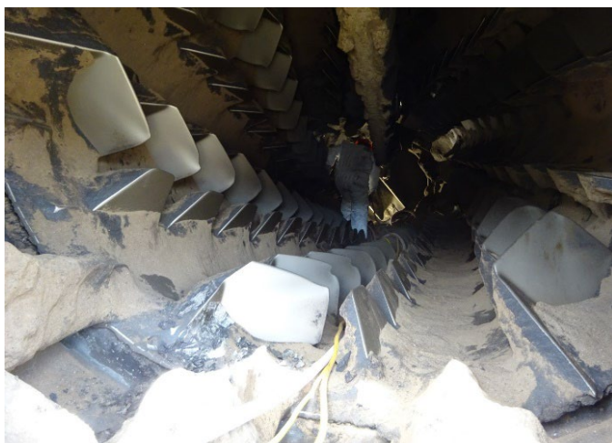
Figure A7. Worker chipping buildup off vanes inside mixing drum located within the yard. Photo by NIOSH.
