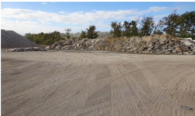
Figure A1. Yard area where roll-off container truck operator dumps reclaimed asphalt and concrete rubble collected from road-side asphalt and concrete tear-out operations. Photo by NIOSH.
