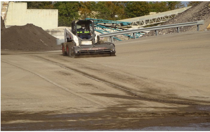
Figure A11. Yard sweeping using the rotary broom with water-based dust suppression attachment on a skid-steer machine. Photo by NIOSH.
