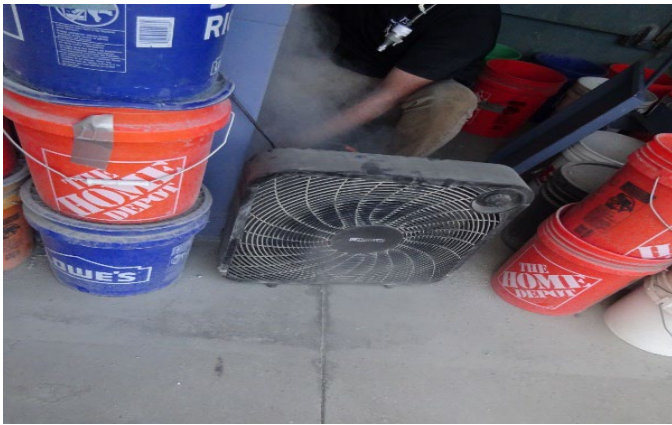
Figure A3. Laboratory QA/QC technician using compressed air to clean out a rock shaker machine. A small box fan was used to try and remove dust generated during cleanout. Photo by NIOSH.
