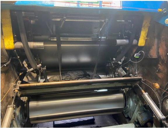
Figure A5. Calender machine bottom bite. Photo by NIOSH.
