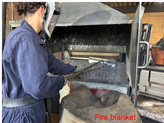
Figure B6. A fire blanket is used to cover the barrel containing cooling copper jackets to emit less smoke than the open barrel with the elephant trunk or the barrel with a metal lid. Photo by NIOSH.
