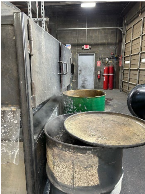
Figure B7. A metal lid is used to cover a barrel containing cooling copper jackets. In this configuration, more smoke was emitted than with the barrel covered with a fire blanket but less than when the barrel was open with the elephant trunk-style hood. Photo by NIOSH.
