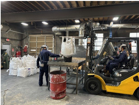
Figure A2. Pouring a super sac containing lead and copper jackets onto the sorting table. Photo by NIOSH.
