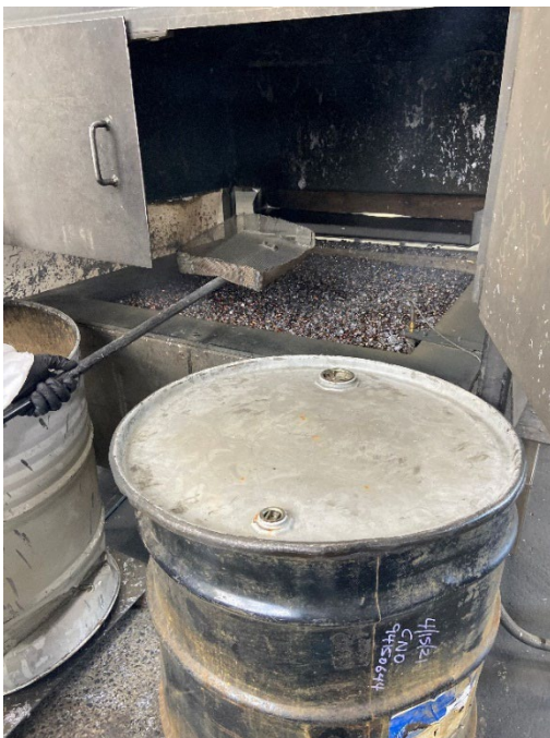
Figure A5. Removing dross and copper jackets from the top of the liquid molten lead inside the furnace. Photo by NIOSH.
