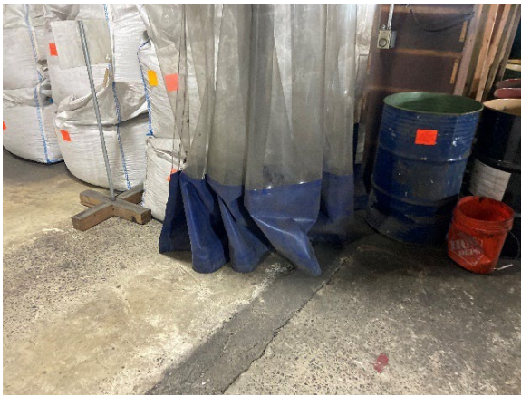
Figure A4. Loose curtain between the main warehouse and the lead melting area, pulled closed while the melting furnaces are powered on. Photo by NIOSH.
