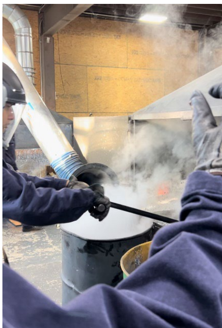
Figure B5. Stationary fume hood with open doors plus elephant trunk-style hood over the barrel, emitting more smoke than when the barrel was covered with a fire blanket or the barrel was covered with a metal lid. Photo by NIOSH.
