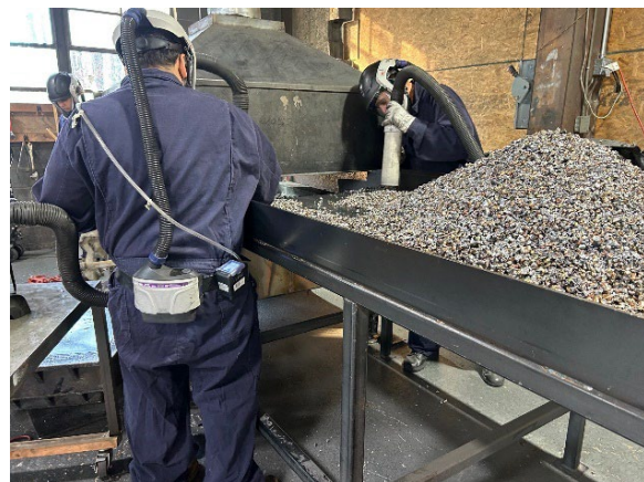
Figure A3. Employees vacuuming rubber from the lead and copper components. Photo by NIOSH.
