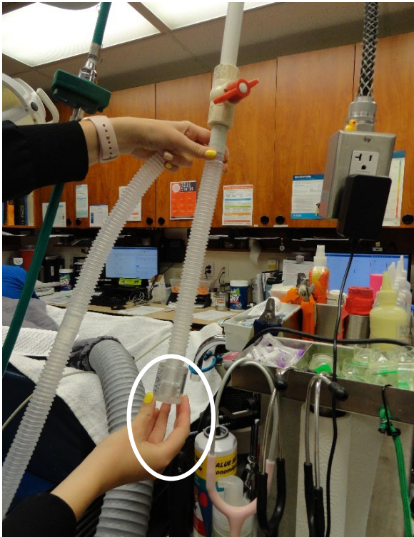
Figure 2a) Veterinary assistant checking function of scavenger system for an anesthesia machine before anesthesia procedure by attaching a tube with a thin strip of flutter paper inside area within the white circle. 2b) Closeup of circled area in Figure 2a) showing the flutter paper elevated from the suction in the scavenger system (see arrow and dashed line). Photos by NIOSH.
