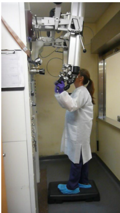
Figure B1. A pharmacist standing on a platform using manipulators on a hot cell to prepare a syringe of radiological isotopes. Photo by NIOSH.
