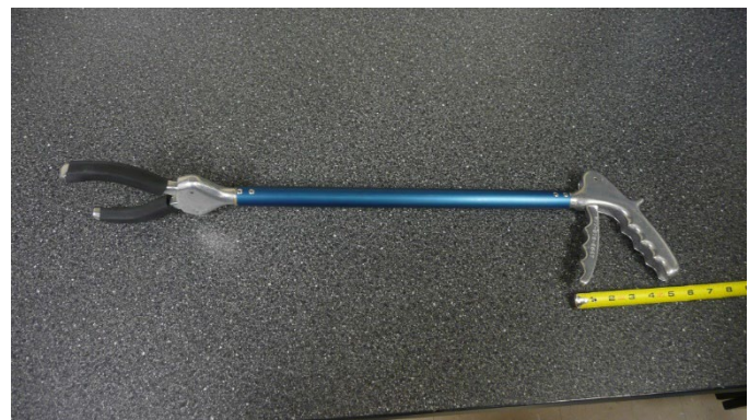
Figure B2. One of the newer remote carrying devices (grabber) used to transport the dose. Photo by NIOSH.
