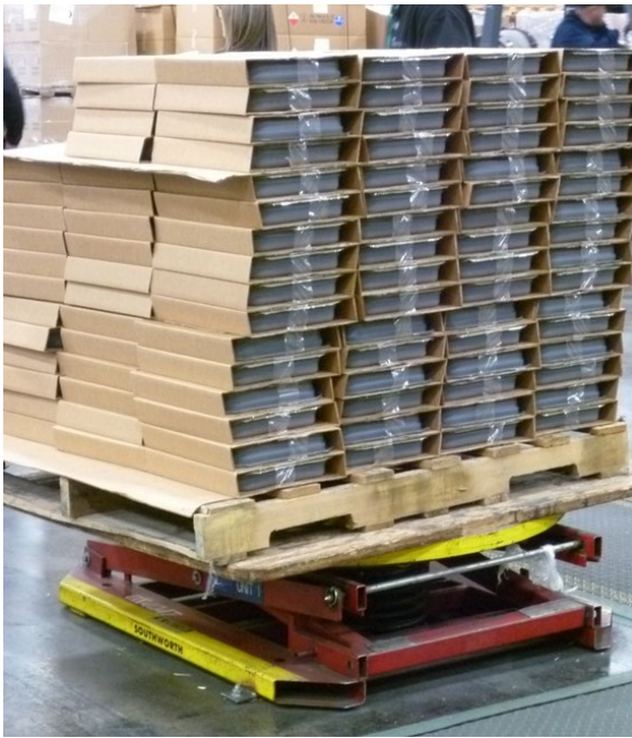
Figure B4. Pallet lift holding about 400 pounds, but lifts are not completely compressed. Photo by NIOSH.
