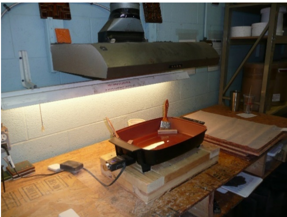
Figure 8. Paraffin wax station, consisting of an electric skillet, a brush, and a roller.
