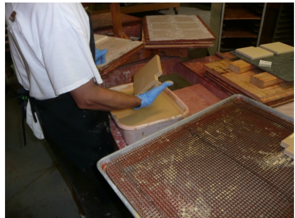
Figure 9. Employee wearing nitrile gloves hand dipping tiles into glaze.
