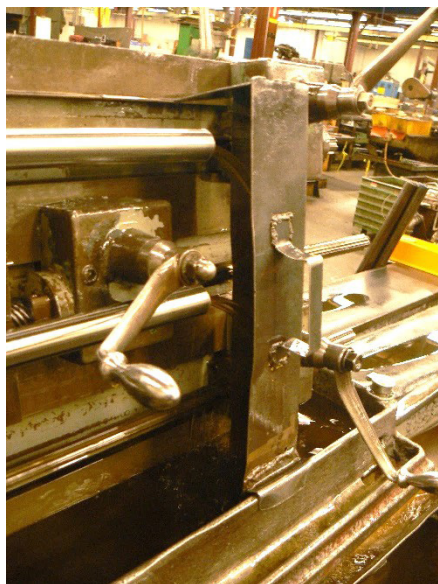
Figure 4. Using the handle, a metal guard is placed over the site on the reaming machine where oil is streaming from the end of metal cylinders. Prior to using this guard, oil splashed from the end of the metal cylinders onto employees.
