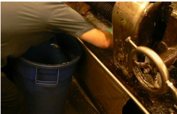
Figure 1. Employee with bare forearms removing metal chips from a drilling machine using his gloved hands.
