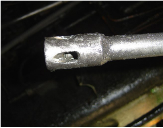
Figure 7. Open tube nozzle with air pressure relief openings along the side. Photo by NIOSH.
