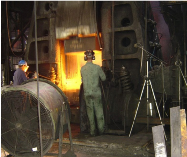
Figure 2. Hammer operator (right) and hammer helper (left) at forge hammer. Photo by NIOSH.
