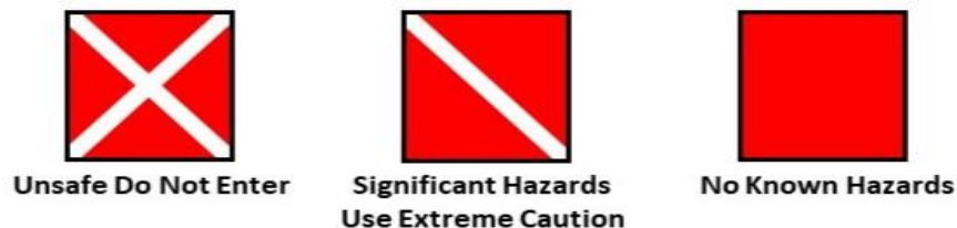
Image 8. IAAI/USFA high-risk building marking system ( Courtesy of USFA )
