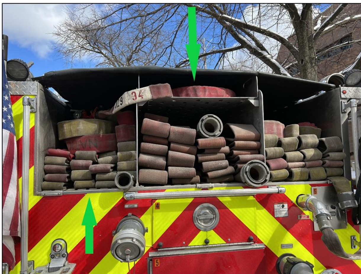
Photo 4. Hose bed on Engine 94. The horseshoe hose load that Engine 94 Nozzle pulled from the engineer's side of Engine 94. The green arrows indicate the hoselines that were pulled. (NIOSH Photograph)
