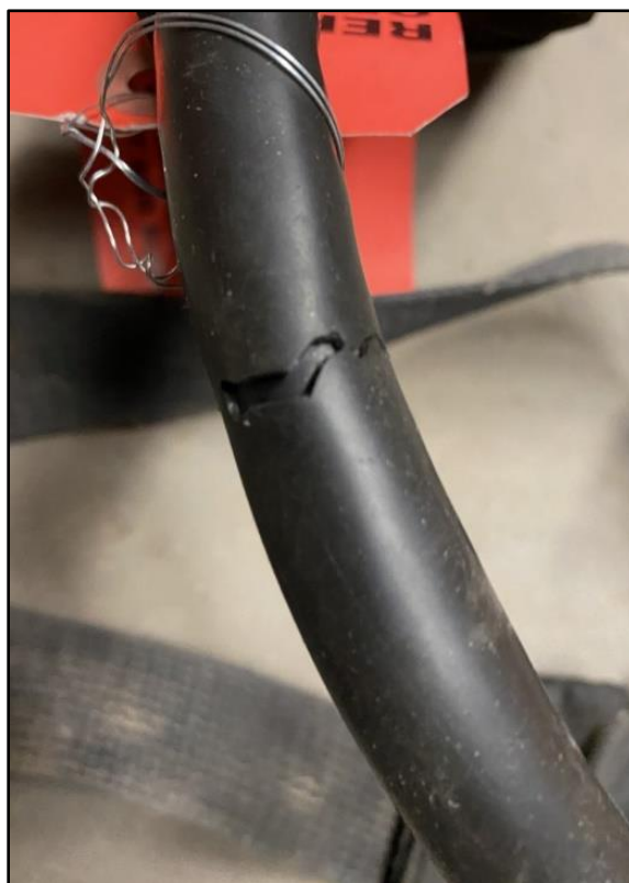
Photo 3. The cracked low-pressure hose with a hole on the SCBA worn by Engine 94 Nozzle. ( Photo courtesy of the fire department. )
