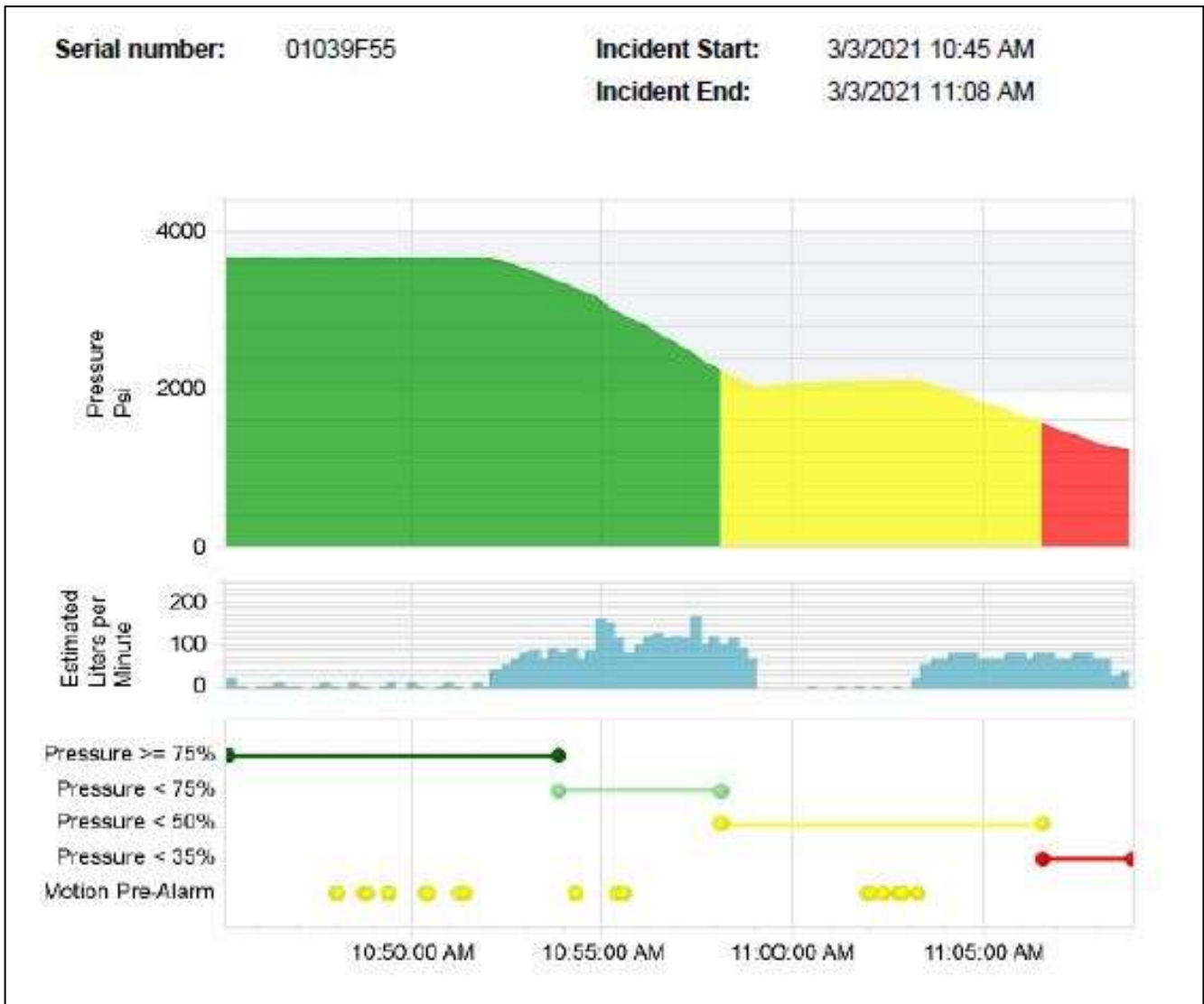
Graph C: Third cylinder on March 3, 2021. Used for culvert tube drill. (Graph by SCBA manufacturer)
