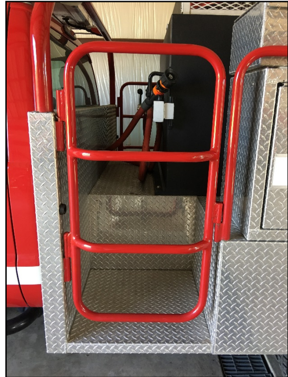
The position on Grass 5-1 that the fire fighter (Fire Fighter “A”) was riding on when he fell off and was overrun by the fire. (NIOSH Photo.)
