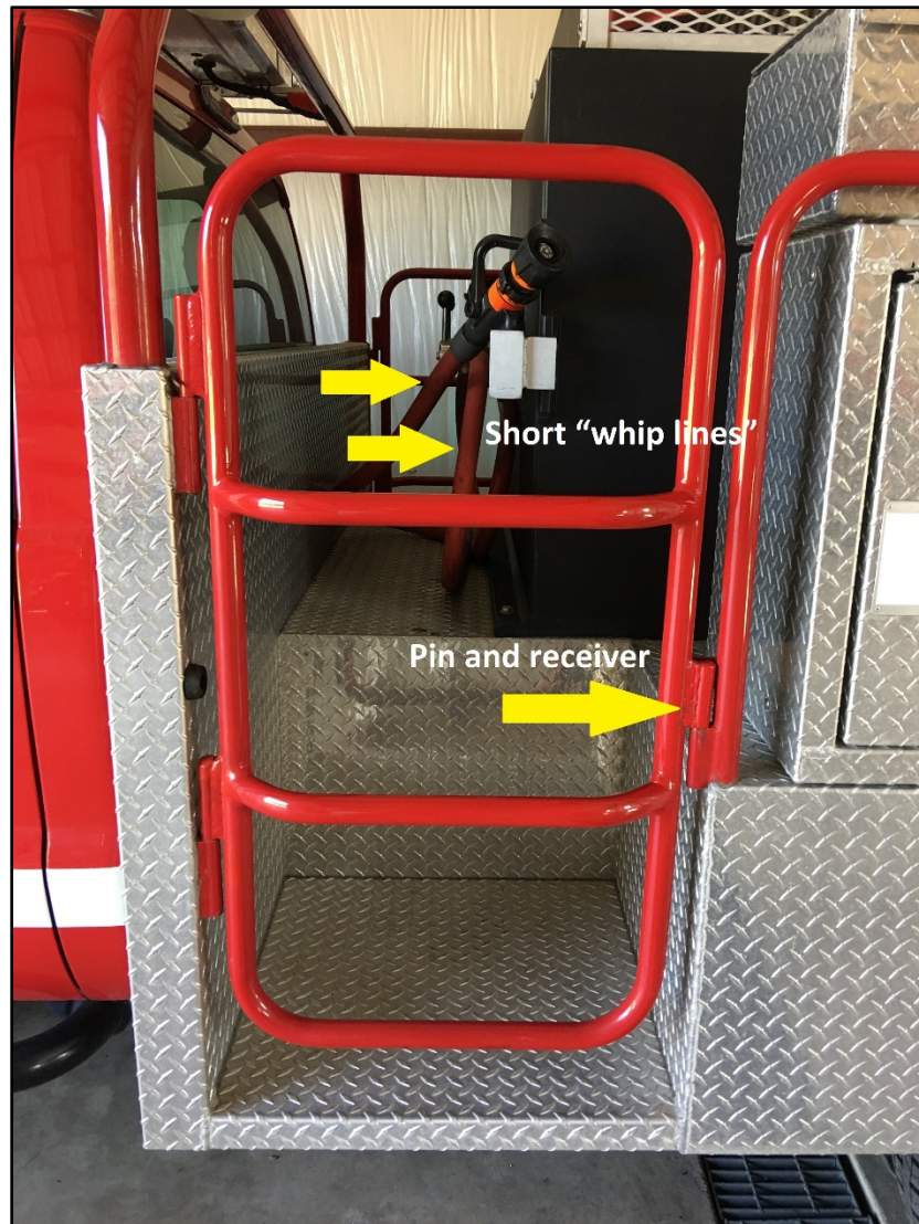
Photo 1. The side step position on Grass 5-1 showing the gate latching mechanism and the short hoselines on each side of the apparatus (NIOSH Photo.)
