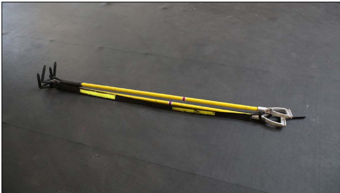
Photo 4. Example of a roof kit similar to the one carried by the fire fighter. A roof kit consists of two six-foot rubbish hooks and a webbed carrying strap weighing a total of 20 pounds.
