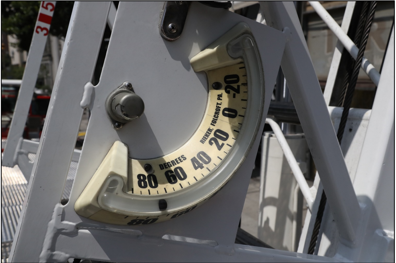
Photo 2. Position of climbing angle indicator for aerial ladder at the time of the incident. (Courtesy of the Fire Department.)
