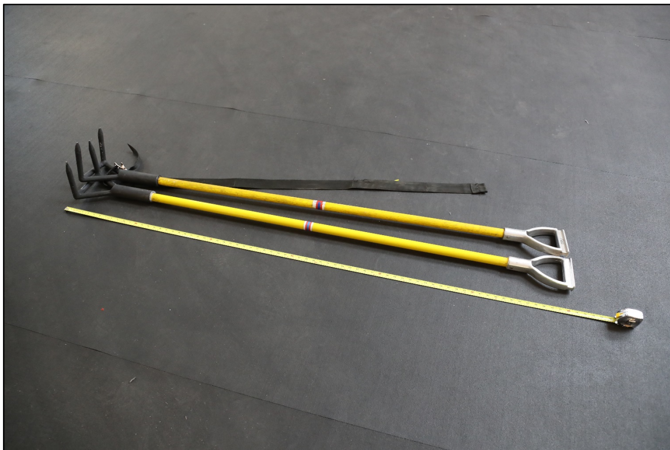
Photo 6. Roof kit (two 6-foot rubbish hooks weighing 20 pounds) carried by the fire fighter. Note the cinch strap for the D handles is missing. (Courtesy of the Fire Department.)
