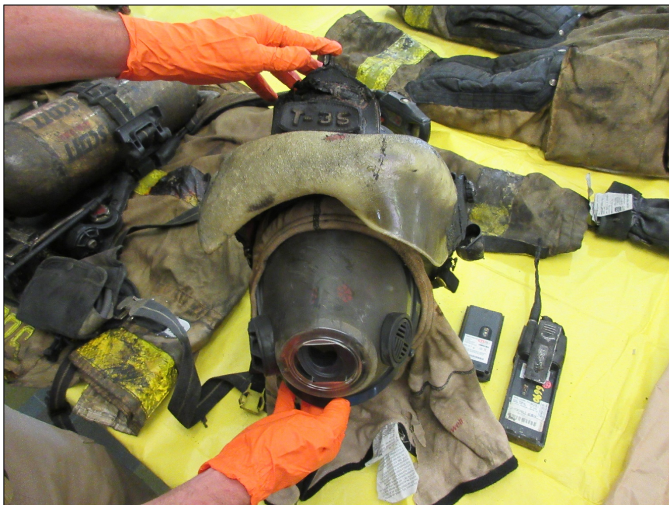
Photo 5. Photo shows thermal damage to the facepiece, helmet and hood worn by the injured Ladder 35 fire fighter. Similar damage has been observed on numerous NIOSH investigations. (NIOSH Photo.)
