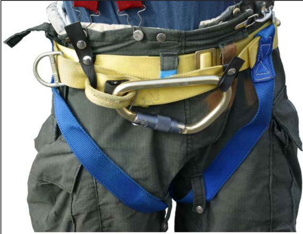
Photo 5. The webbing and carbiner used by the fire department as part of their personal escape system.
