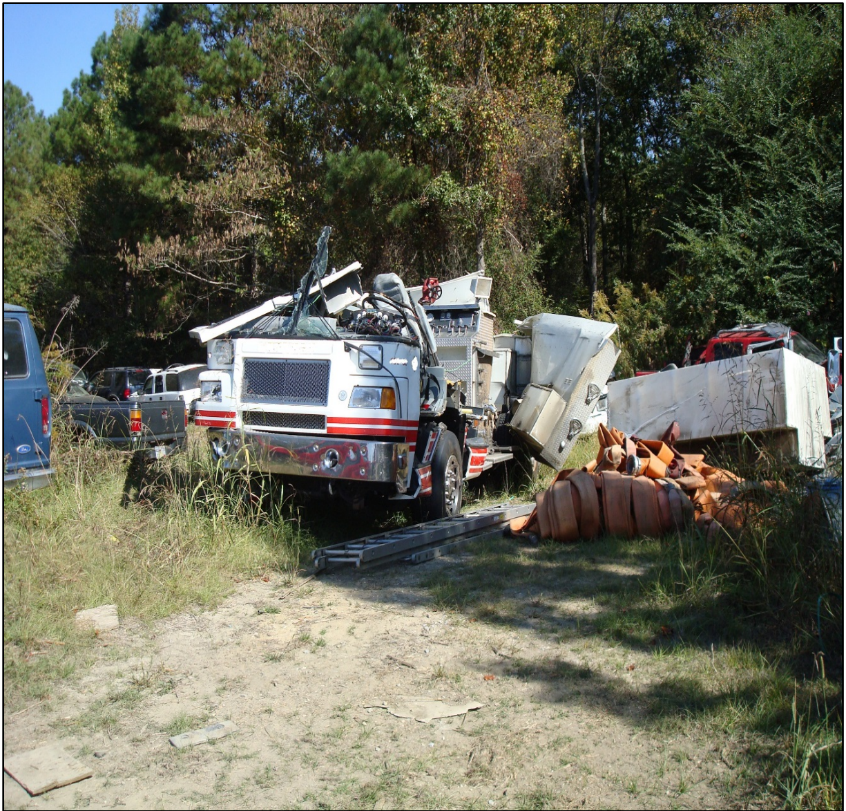
Photo 5. Engine 3 in the locality’s storage facility after removal. Note that the damage shown in photo is not due to extrication procedures, rather from the rollover and end over end flipping. (Photo by NIOSH)
