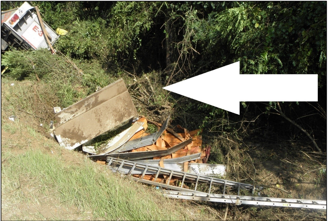
Photo 3. Engine 3’s water tank, hose and equipment that were ejected during the roll over and end over end flip. (Photo courtesy of the fire department)
