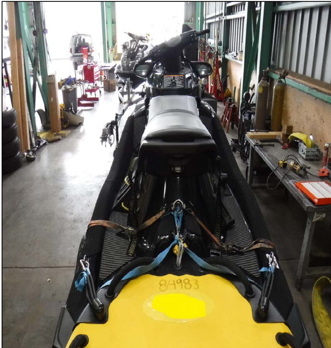
Photo 7. RWC shown with modified connection for the rescue sled attachment. The bow of the rescue sled is attached and riding on the rear of the RWC. The manufacturer of the water craft does not make the rescue sled or the transom attachment.
