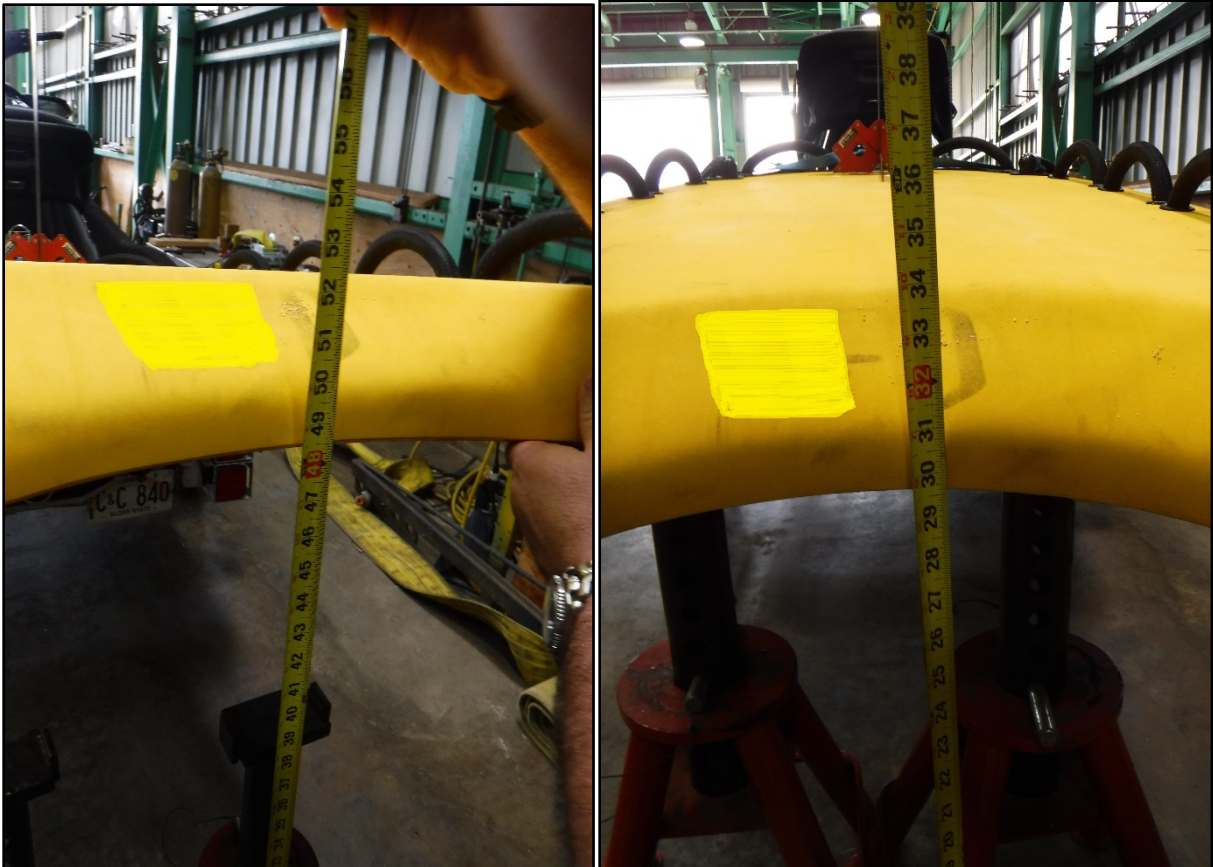
Photos 9b and 10. The connection at the rear of the RWC and the front of the sled prevented side to side but not the up and down motion of the rear. The amount of up and down movement for the rear of the rescue sled was 18 inches. Photo 10 on right measures distance of rear of the rescue sled to a level running position and Photo 9b on left shows the level of rise is approximately 18 inches from a level running position.
