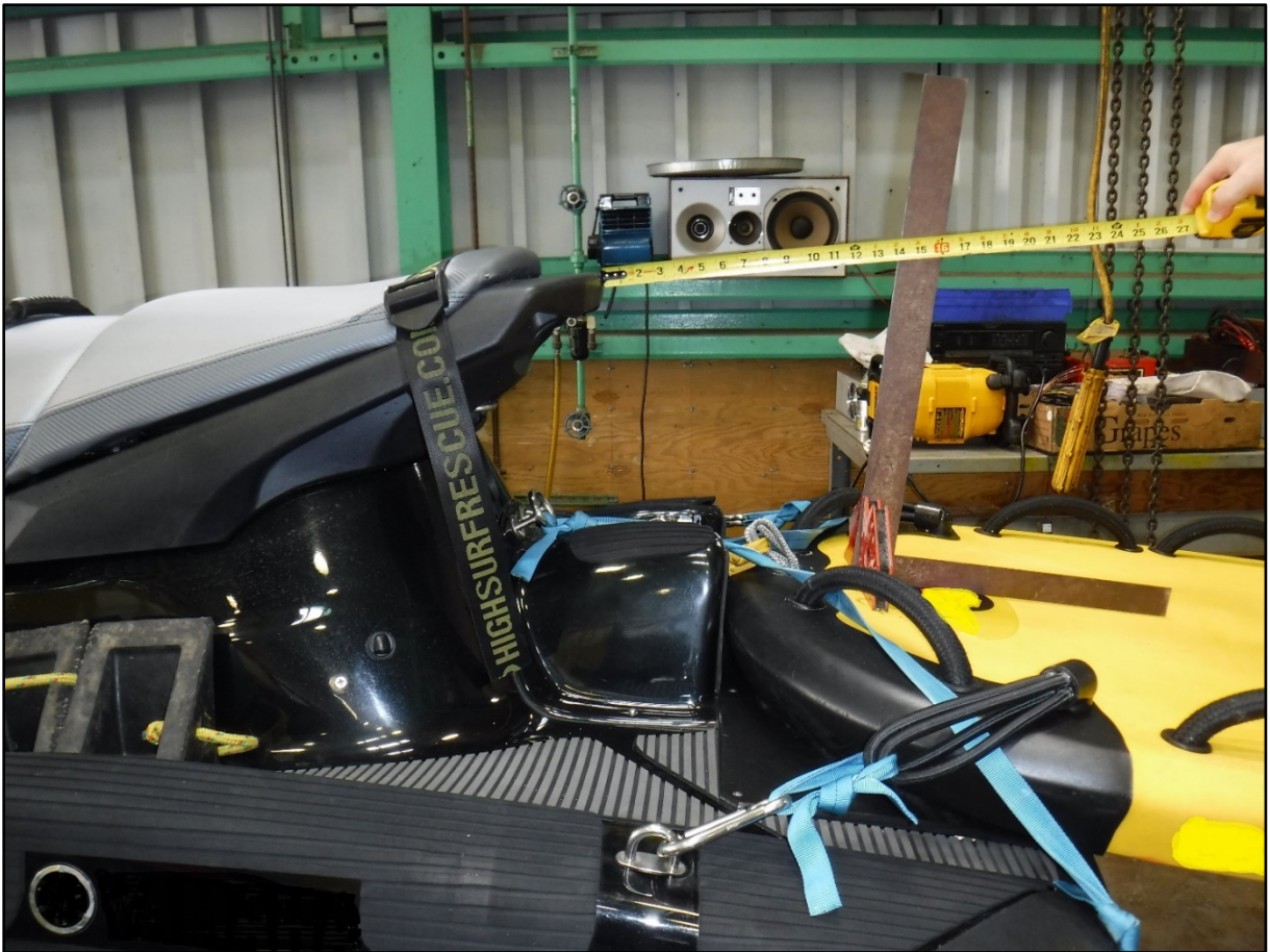
Photo 8. Sled orientation to rear grab bar where the victim likely struck his head. This distance is measured at approximately 14 inches with the rescue sled in the downward orientation and decreases to 8.5 inches as seen in photo 9. Riding prone on the rescue sled has many disadvantages for the swimmer with the main disadvantage of the swimmer being thrown forward or forward inverted (the slang term for this is being scorpioned), and striking the rear of the RWC.
