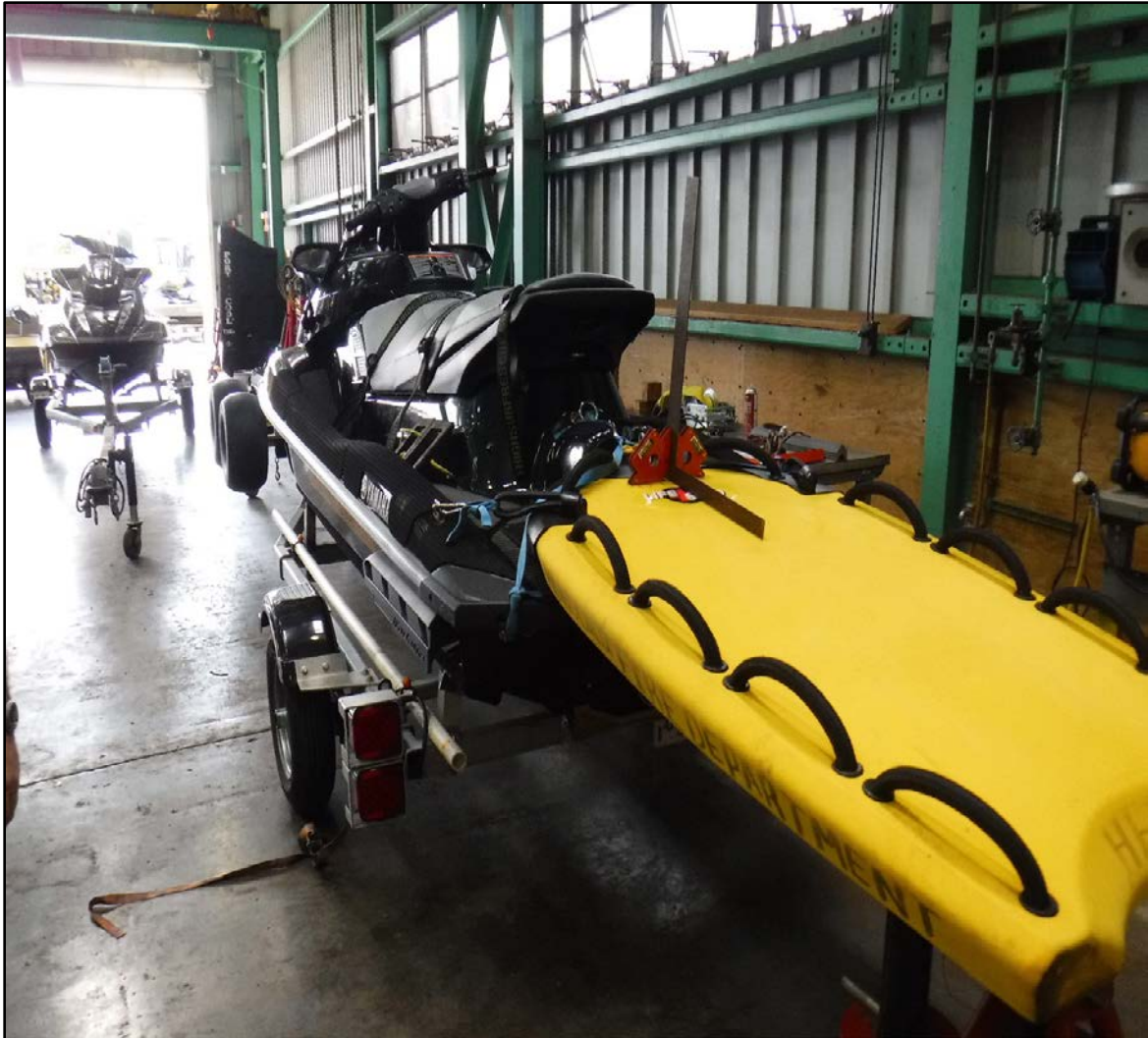
Photo 6. Rescue Water Craft (RWC involved in this incident ) with rescue sled attached and oriented in the use position. (Photo courtesy of fire department)
