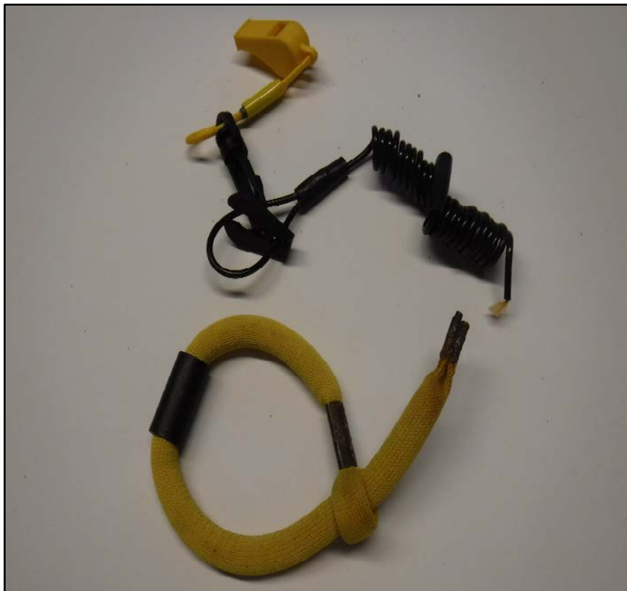
Photo 13. Most personal watercraft are equipped with a safety lanyard that either kills the engine or throttles the watercraft to neutral so operators who may have fallen off can re-board without the watercraft driving away. This watercraft had a safety lanyard that failed due to hidden corrosion underneath the outside covering. This photo shows the corroded area where the lanyard break occurred. The second time the RWC driver jumped in to help the fire fighter who fell off the sled, the RWC kept motoring away from them because the lanyard key stayed in the safety switch and the wristlet stayed on the operators wrist. (Photo courtesy of the fire department)
