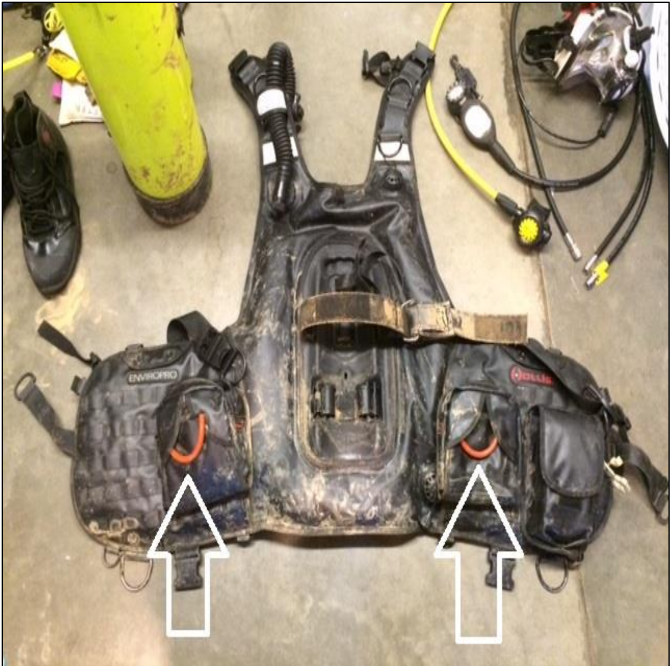
Photo 8. Photo of Diver 4's buoyancy control device (BCD) vest showing ditchable weight release pull handles. (Photo by NIOSH.)
