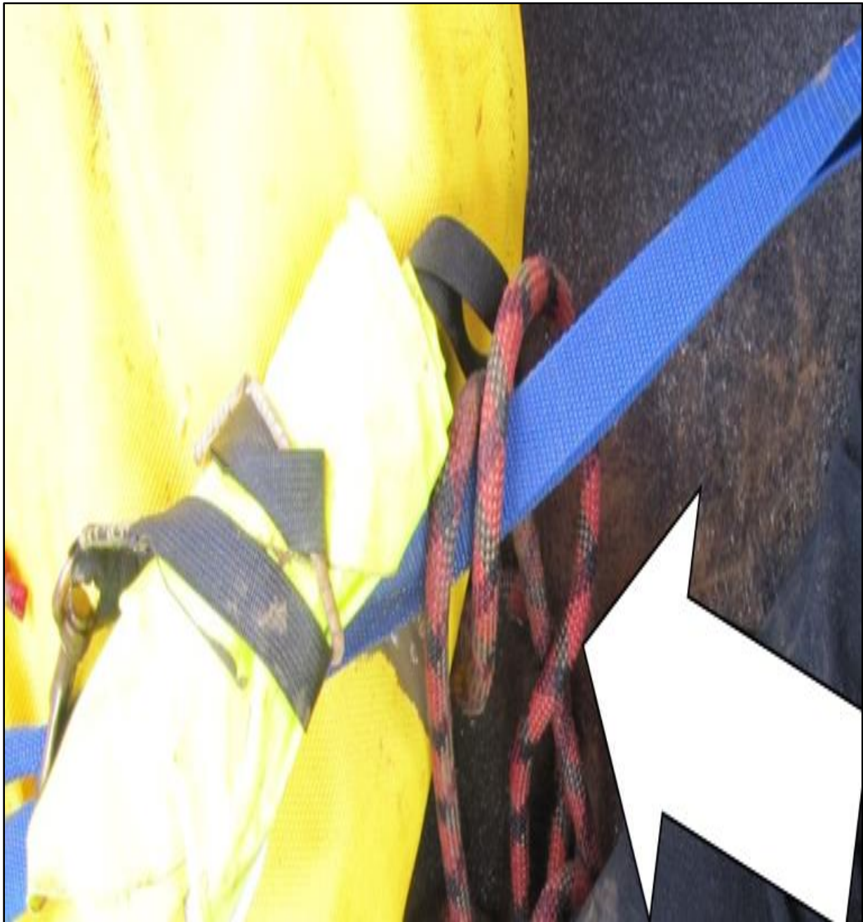
Photo 2. A 158 foot, 7/16 th inch search rope tangled up around the lift bag attached to the victim. The other end had a D-ring closure and was attached to the cage. A mutual aid diver cut the rope before recovering Diver 4.
