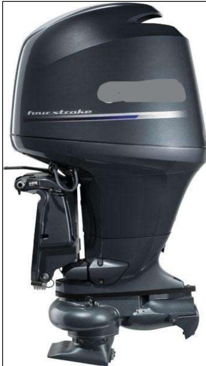
Photo 11. Example of a large horsepower outboard jet drive engine ( Photo courtesy of Bing images. )
