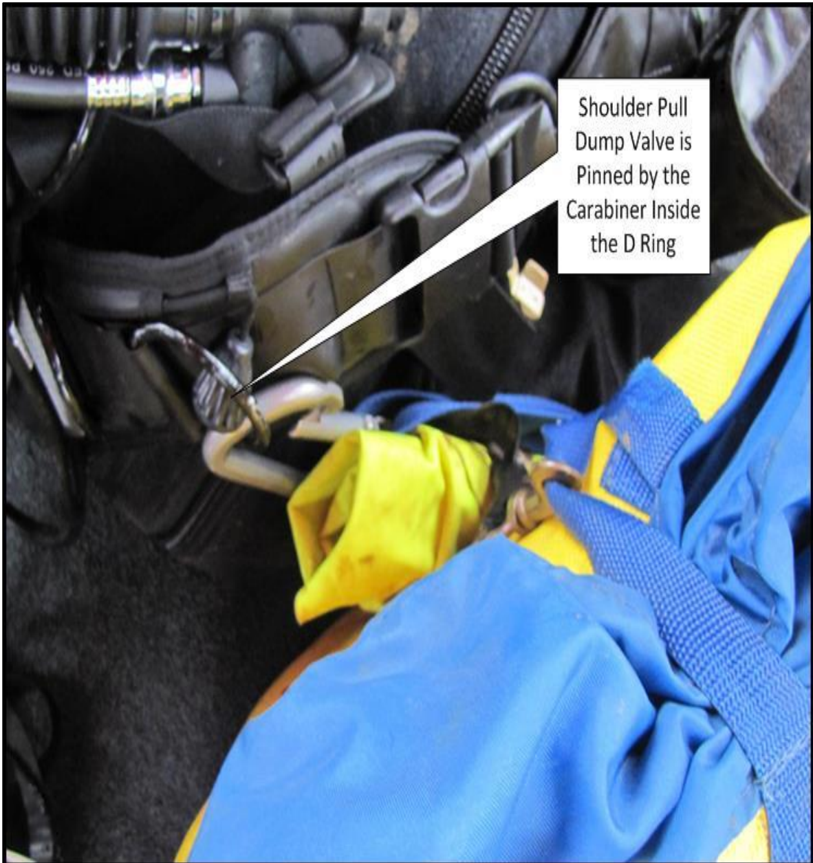
Photo 1. Close up photo taken when the victim was recovered showed his shoulder dump valve was possibly pinned “open” by the body bag carabiner inside the D ring. This could have made maintaining positive buoyancy difficult as any air pushed into the BCD may have escaped here.
