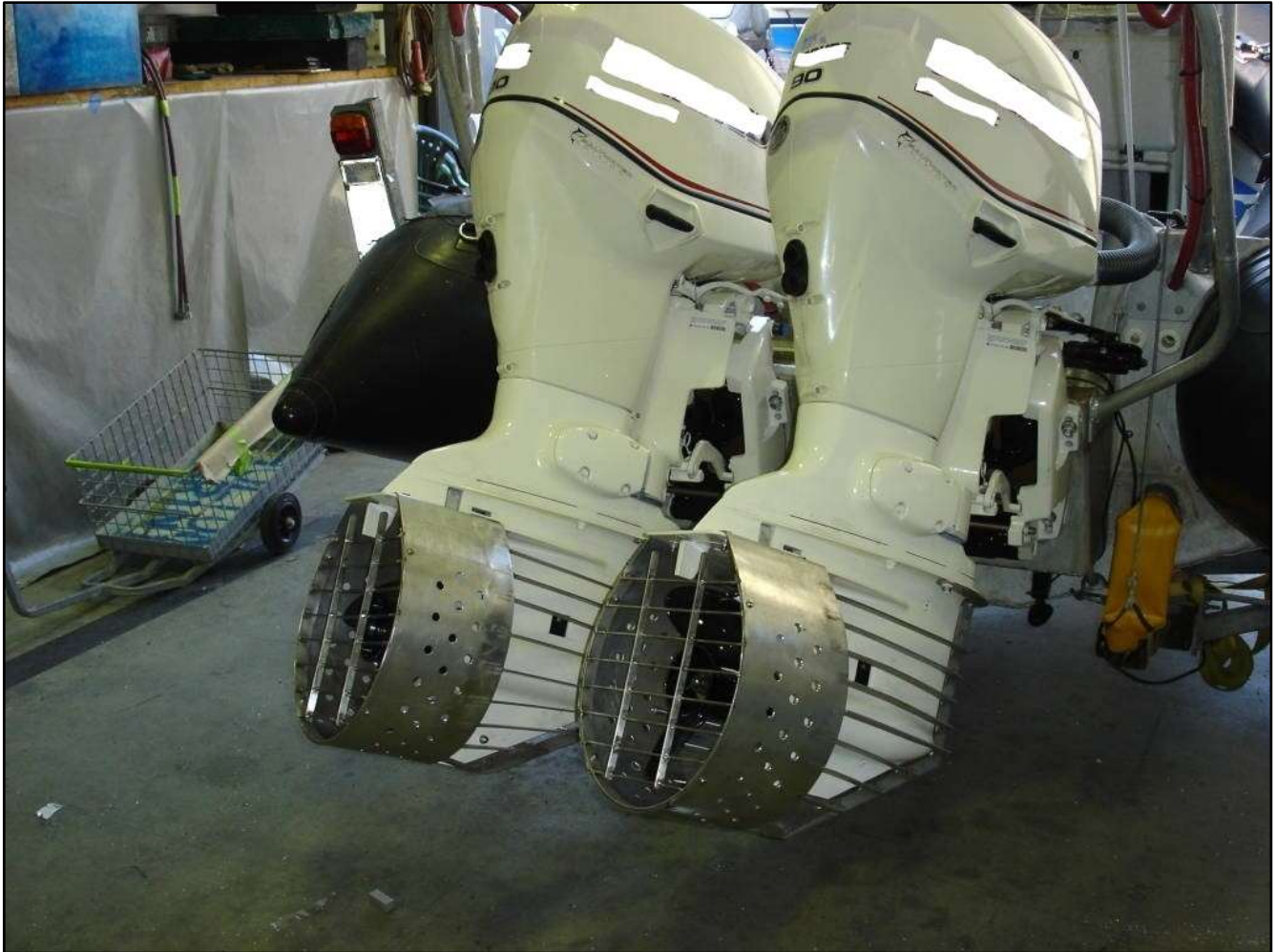
Photo 10. Example of propeller guards on larger twin outboards ( Photo courtesy of Bing Images/Holtonmarine. )
