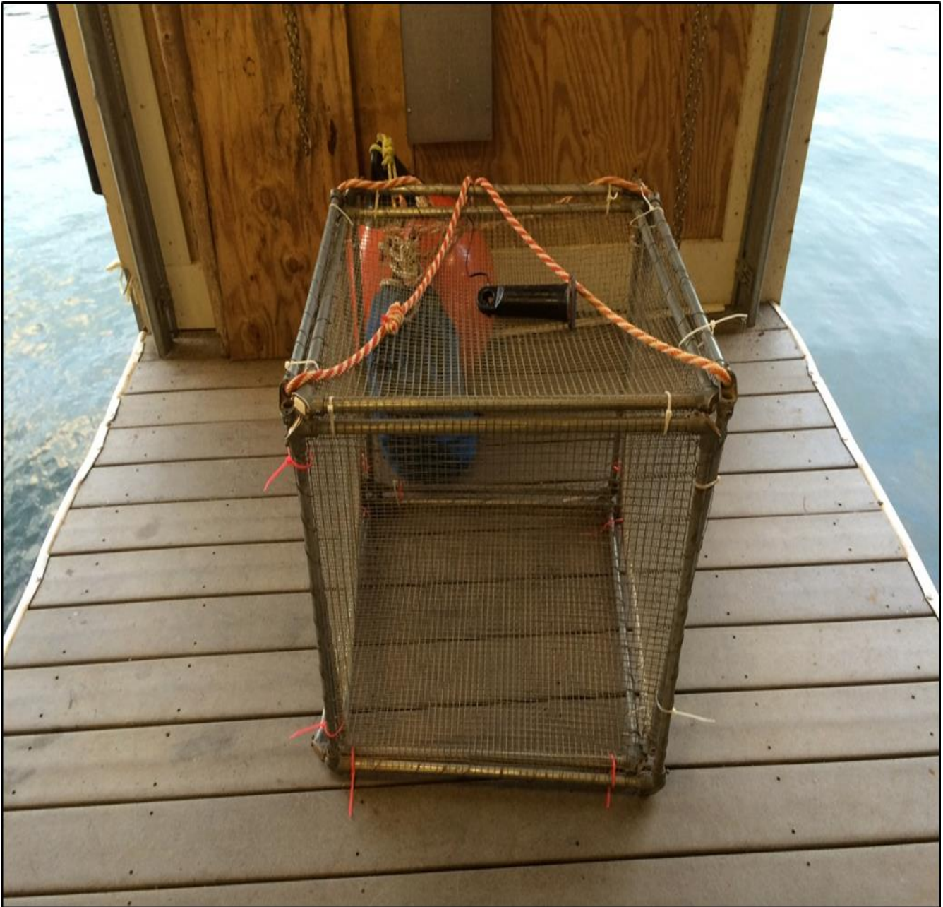
Photo 6. The “cage”. It is used to anchor the ascent/descent rope to the bottom and is the point of reference for sonar and divers when performing searches. Its metal construction and form provide a distinguishable target for the sonar operators. Once positioned, it can be later moved by surface boats with sonar closer to the “target” to reduce blind diving. (NIOSH Photo.)
