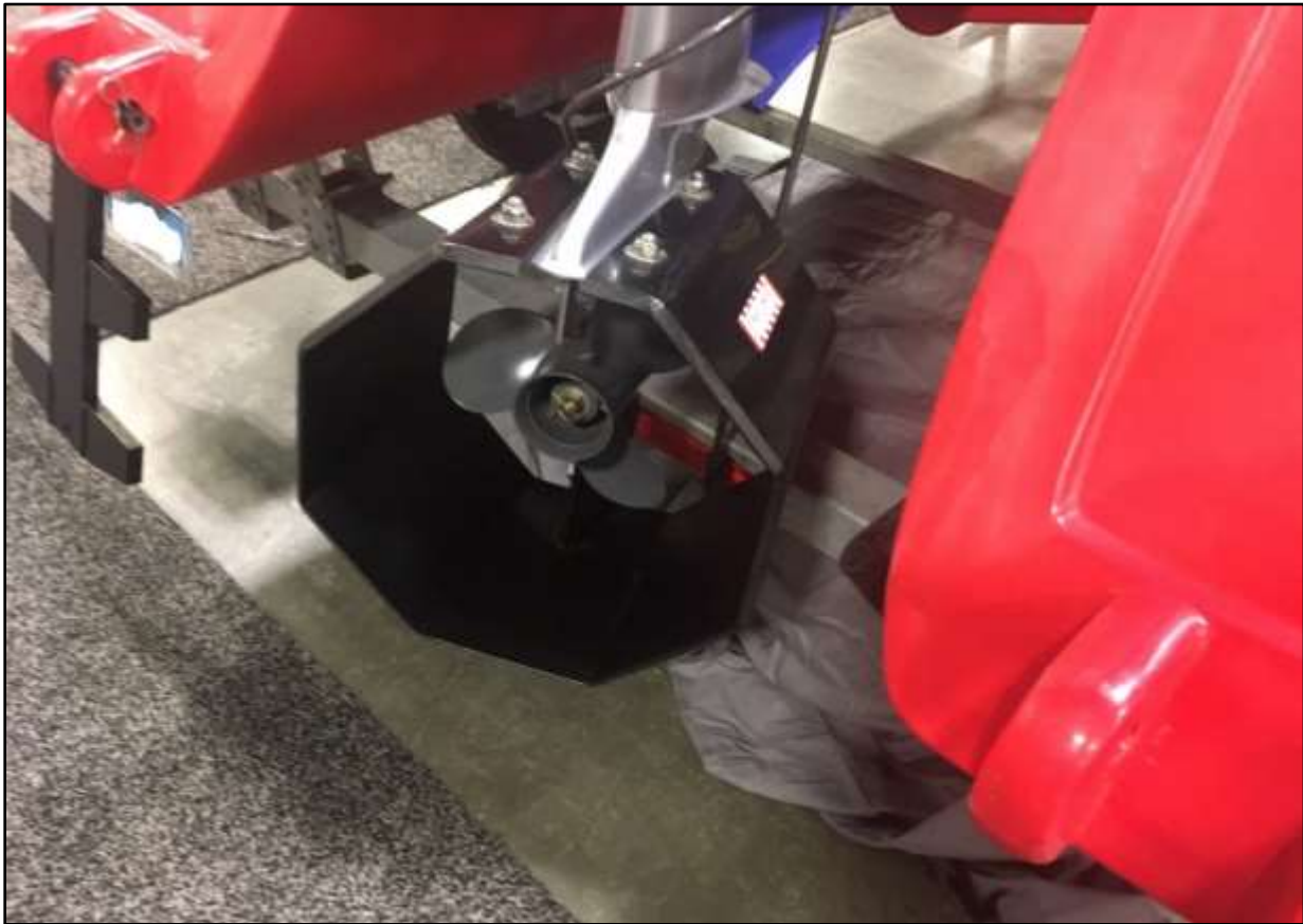
Photo 9. An example of a propeller guard for a small and medium sized outboard engine. There are also jet drive propulsion options for outboard engines ( Photo by NIOSH. )
