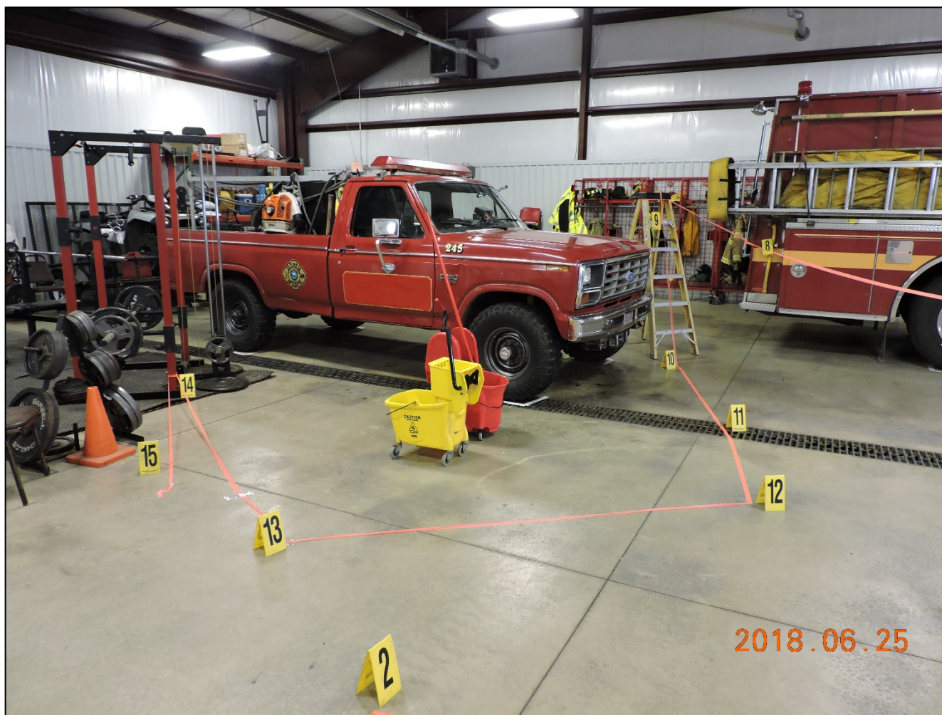
Photo 10. Photo shows estimated travel path (estimated by State Fire Marshal’s Office investigators and County Sheriff’s Deputies) of the cylinder after it struck the rear corner of Engine 22 (point 8), then struck the fire fighter at approximately Point 9 before falling to the engine bay floor (point 10) and expending energy as it moved across the engine bay floor before coming to rest at Point 15 near the exercise weight equipment. Also see Photo 8 and Photo 9. Photo courtesy of State Fire Marshal’s Office.
