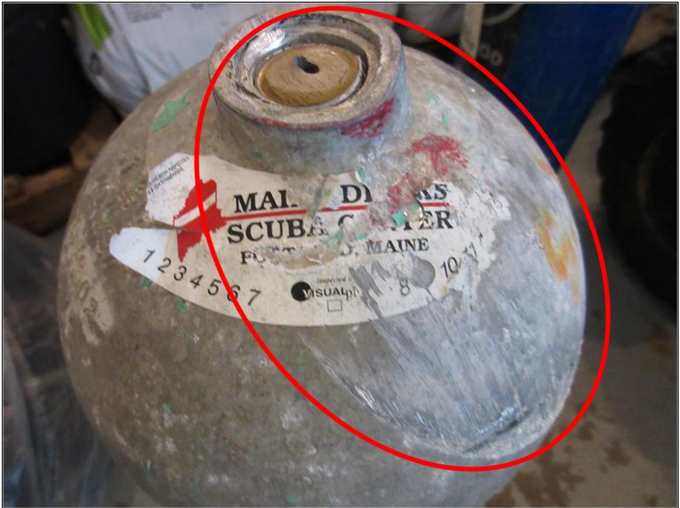
Photo 4. The SCUBA cylinder involved in this incident. Note the scuff marks on the cylinder caused by the cylinder striking the engine bay wall (see Photo 2 and Photo 3). The area highlighted in red is the area that impacted the wall.
