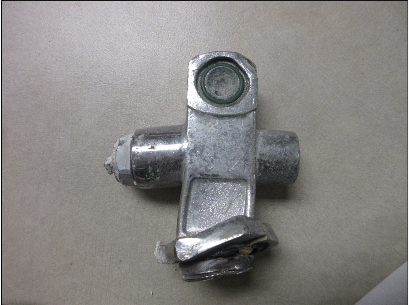
Photo 5. SCUBA cylinder valve involved in the incident. This cylinder valve was broken off from the SCUBA cylinder when the cylinder struck the engine bay wall. It is believed that the valve handwheel (left side of valve in Photo above) also broke off when the cylinder struck the wall. See Photo 4.
