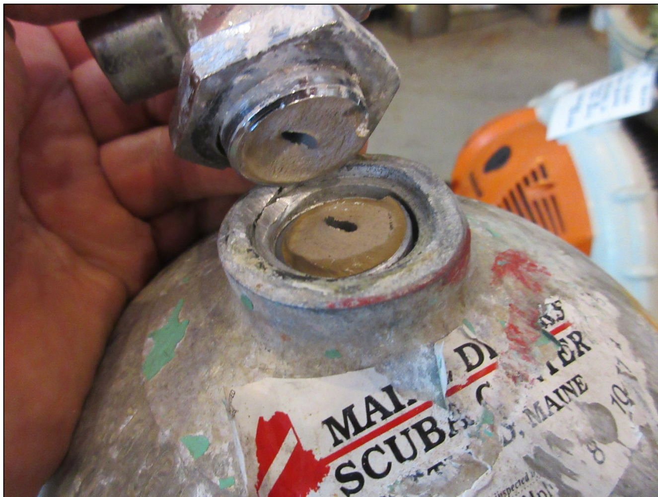
Photo 6. Photo shows how cylinder valve broke off the SCUBA cylinder when the cylinder impacted the engine bay wall. Also see Photo 2, Photo 3 and Photo 4. NIOSH Photo.
