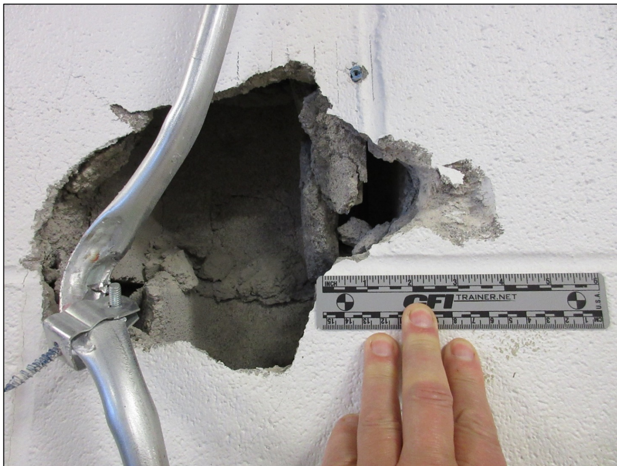
Photo 2. Hole in engine bay wall caused by SCUBA cylinder (valve end) striking the wall after the cylinder became a projectile.
