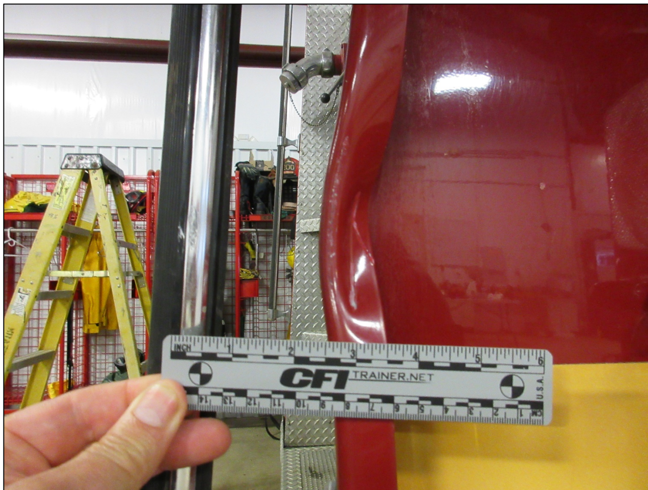
Photo 7. Close-up view of the dent on the rear of Engine 22 (officer side) where the pressurized cylinder struck the engine before glancing off engine and striking Fire Fighter 2. NIOSH Photo.
