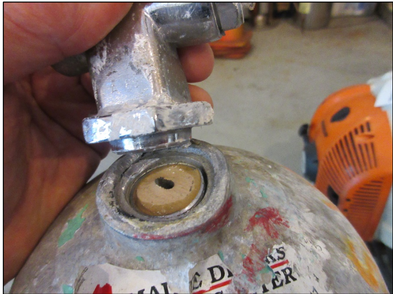
Close-up photo shows broken cylinder valve and neck area of SCUBA cylinder that struck the 33-year old fire fighter. (NIOSH Photo)
