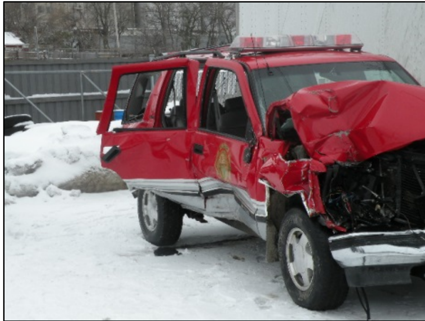
Photo 3. The damage to Utility 105 caused by the crash and the extrication of the two fire fighters. (Photo courtesy of the fire department)
