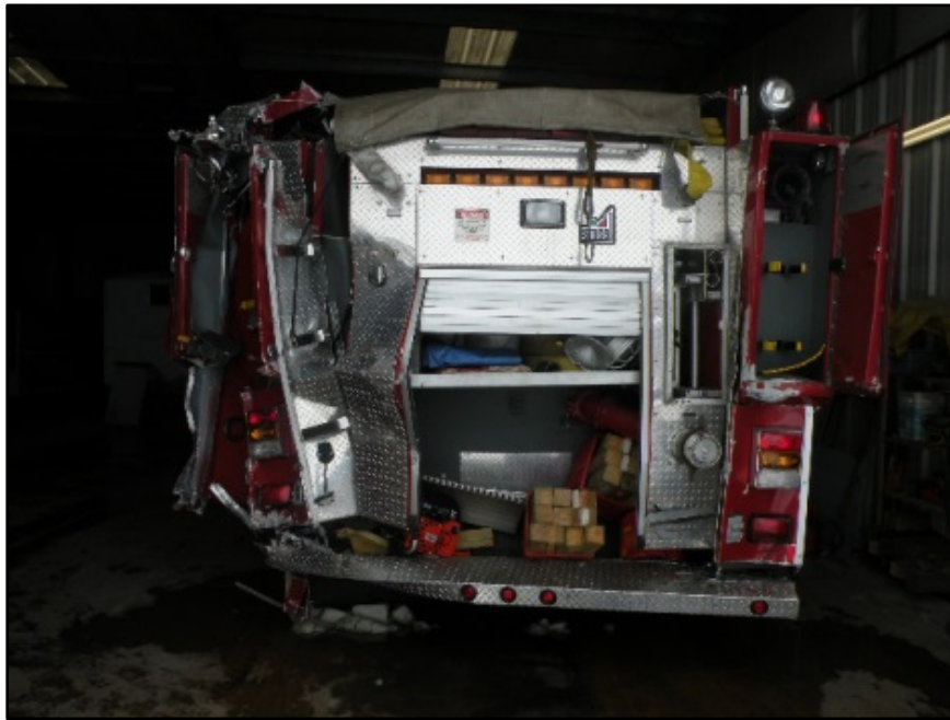
Photo 2. The extensive damage to Engine 102 after being struck by the car hauler on the interstate. This picture was taken the next day at the towing company where Engine 102 was stored. (Photo courtesy of the fire department)
