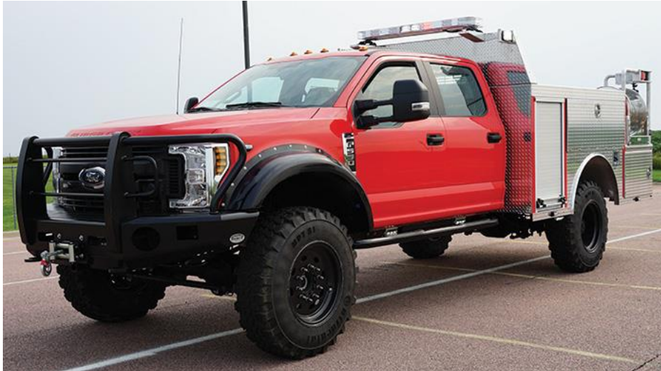
Image 1. Example of a Type 6 Wildland Fire Engine (Fire Apparatus & Emergency Equipment Staff, 2019).
