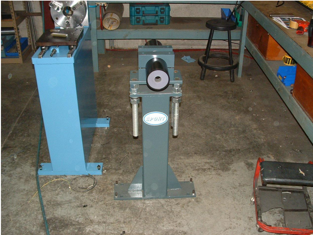
Photo 9. Sleeve bearing-style support system for extended bar stock engineered by J.F. Berns
