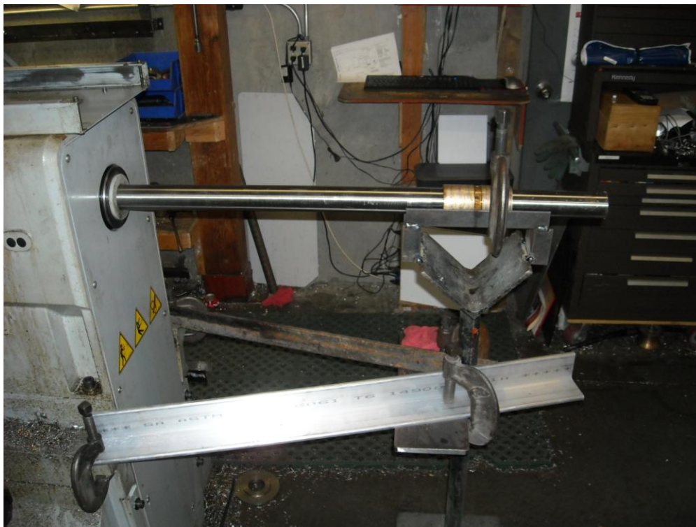
Photo 8. Shop-built support system for supporting extended bar stock
