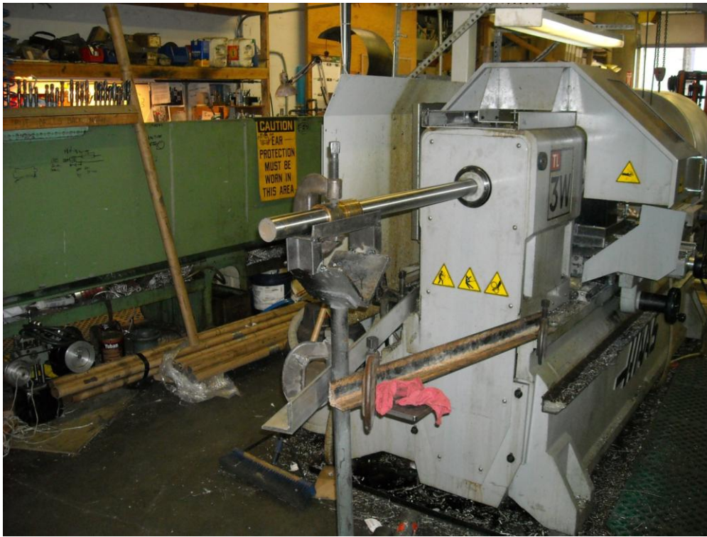
Photo 7. Shop-built support system for supporting extended bar stock
