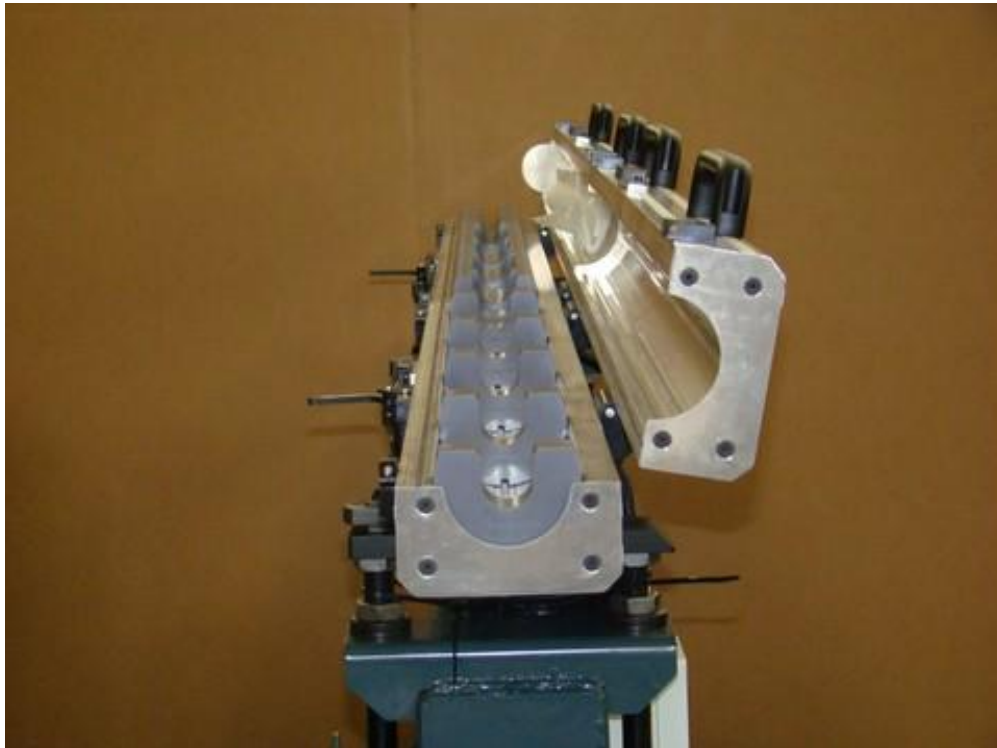
Photo 10. Cradle-style support system for extended bar stock engineered by J.F. Berns
