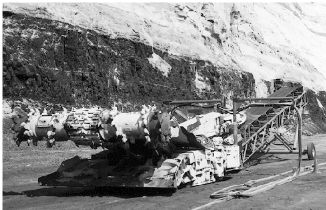
Figure 5.—JOY 12CM with stacking conveyor as used in OP experiments.
