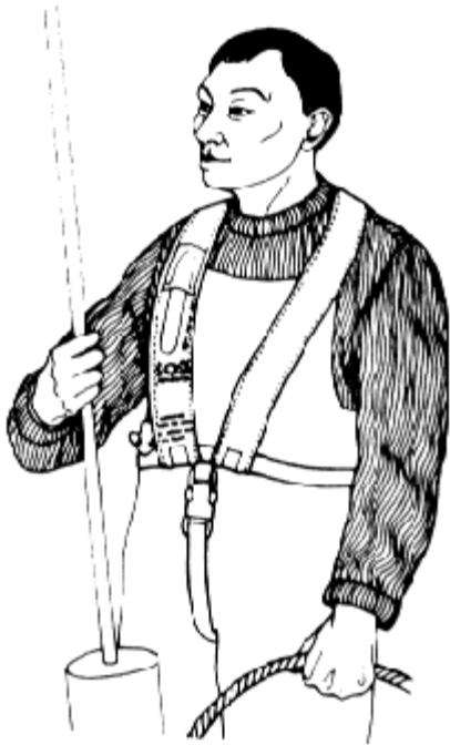
Figure 11: Suspenders (uninflated)–not USCG approved. (Source: ASGCP [1992]. Reprinted with permission. Drawing by S. Laurie.)
