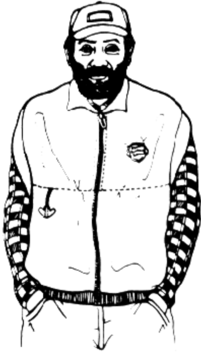
Figure 5: Type V hybrid PFD. (Source: ASGCP [1992]. Reprinted with permission. Drawing by S. Laurie.)
