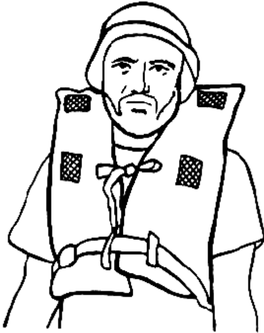
Figure 7: Type II PFD nearshore buoyant vest. (Source: ASGCP [1992]. Reprinted with permission. Drawing by V. Culp.)
