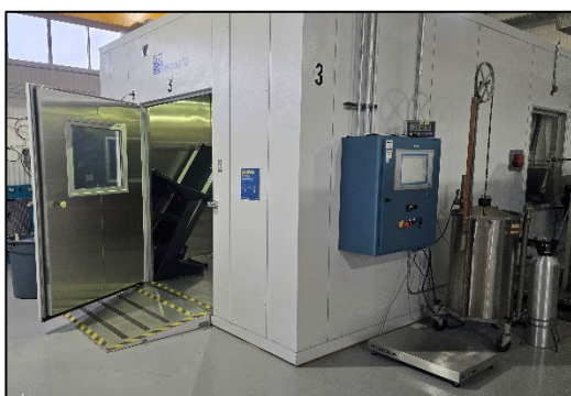
Figure 2-12. Outside view of NIOSH environmental conditioning chamber
