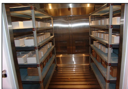
Figure 2-13. Inside view of NIOSH environmental conditioning chamber
