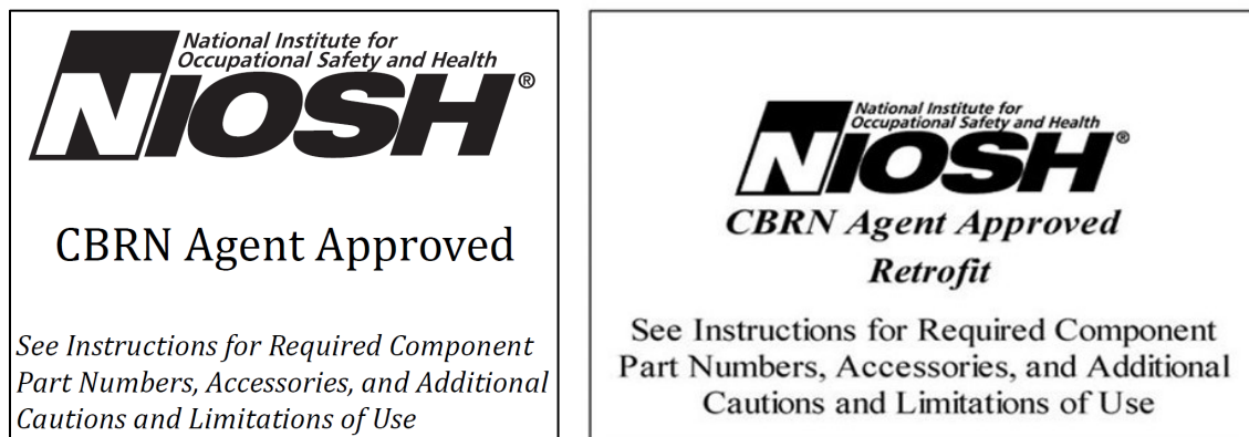
Figure 3-5. NIOSH “CBRN Agent Approved” label (adhesive) for new and retrofitted CBRN SCBA
