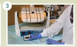
Remove one plate at a time. Strictly control the time from stopping mixing to reading the plate to 1, maximum 1.5 minutes. Make sure that you treat all plates the same (±10 sec).
