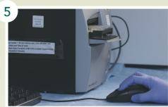
Read the plate at 590 nm. After reading each plate, save results.
