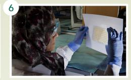
Review the calibrator plate and the sample plates for contamination, leaking, dark color, or abnormal volume. If confirmed as random occurrences, mask the wells.
