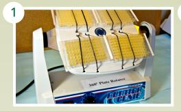
After 42 hours of incubation, remove plates from the incubator and place them into a 360 degree orbital mixer for 30 min. During this time the plates cool down to room temperature and mix thoroughly.
