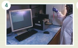
During this minute, wipe the plate bottom to remove any particles or dust, open the sealing membrane carefully to prevent liquid spilling, and place the plate into the plate reader. Gently fan the air above the plate to remove micro-bubbles.
