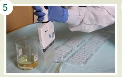
Add 200  $\mu$ L growth medium to all plates using a 12-channel electronic pipette (50–1,250  $\mu$ L) with the repetitive pipetting function and volume set to 200  $\mu$ L.
