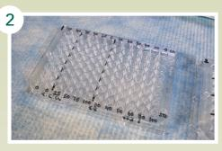
Plate #1 is used for the calibrator with 8 replicates/concentration. Write the volumes of sodium ascorbate (SA) at the top of each column and the volumes of calibrator (CAL) at the bottom of each column.
