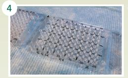
To help with the correct transfer of diluted samples into the plate, divide the plate into columns and rows. Each sample will occupy four wells. Label the sample # on the plate.
