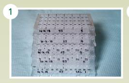
Label each plate on the front with the date and analyst initial. Write the plate number on the upper left corner and on the front.
