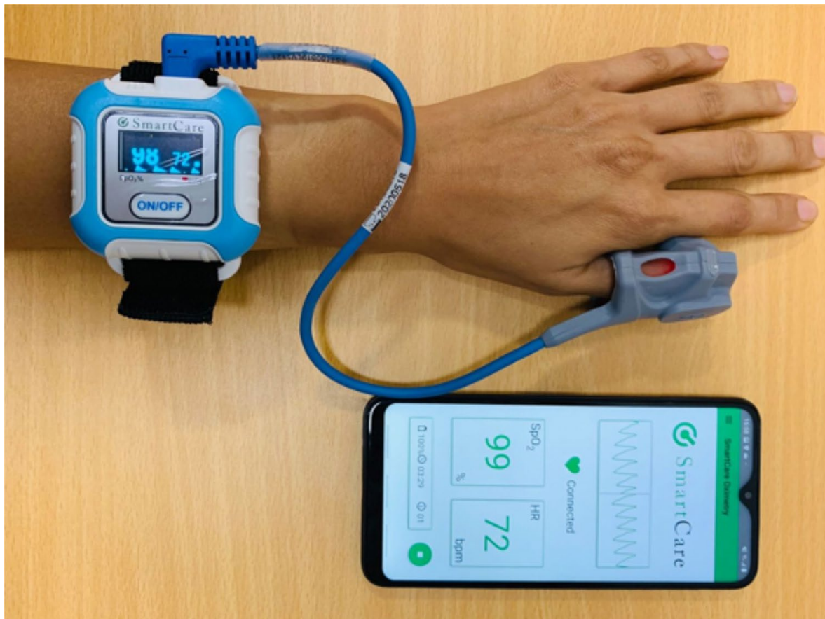
Appendix Figure. Wearable pulse oximeter device and smartphone display used for remote patient monitoring for monkeypox virus infection in 2 female travelers returning to Vietnam from Dubai, United Arab Emirates, 2022. The wearable device reduces clinical staff contact with patients.
