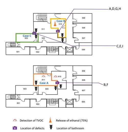
**Appendix Figure 1**. Layout of floors 5 and 6 of a quarantine hotel in Taipei City, Taiwan, December 2021, showing the relative locations of the tracer-gas experiments. Symbols indicate where investigators released ethanol (75%), location of the bathrooms, and where tracer gas was detected.
