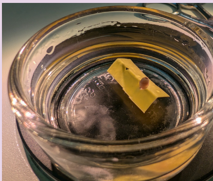
Figure 3a The simple support allows you to orient the fly larva with the head down and posterior segment facing up toward the microscope lens.
