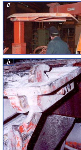
(a) Bolter canopy with rounded edge. (b) Clamps hold the screen in place while the ATRS is raised against the roof, then retracts automatically.
