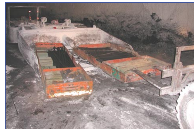
Scoop bucket loaded with pods of bolting supplies for the MHS.
