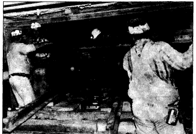
Figure 12.—Miners using timber car to raise 39-kg (85-lb) rail for roof support in an eastern Ohio coal mine.
