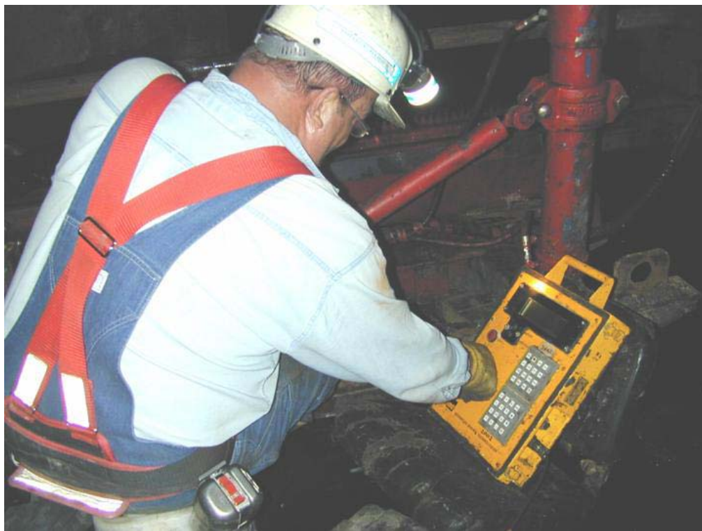
Figure 18. Target Drilling Engineer performing survey of borehole using DDM MECCA unit.
