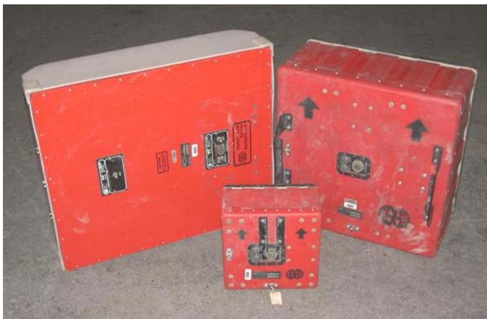
Figure 6. Photo of 200- (antenna size 24 in by 24 in), 300- (antenna size 27 in by 31 in) and 400-MHz antennas (antenna size 12 in by 12 in).
