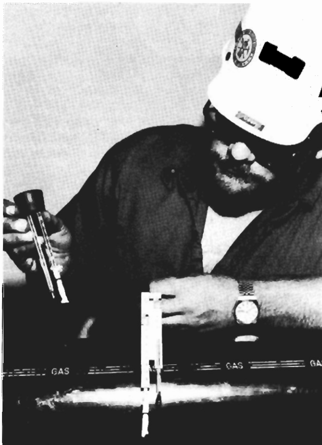
FIGURE 2. - Relative humidity and temperature being measured with psychrometers.
