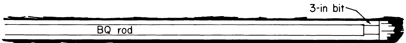
FIGURE 4. - Modified drill string with 3-inch bit.
