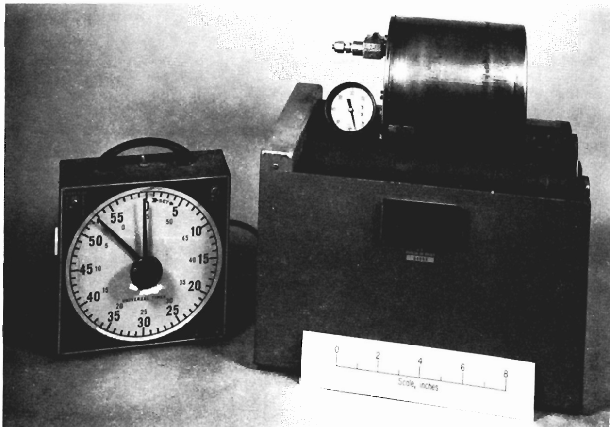
FIGURE 7. - Roller machine for tumbling coal samples in ball mill.
