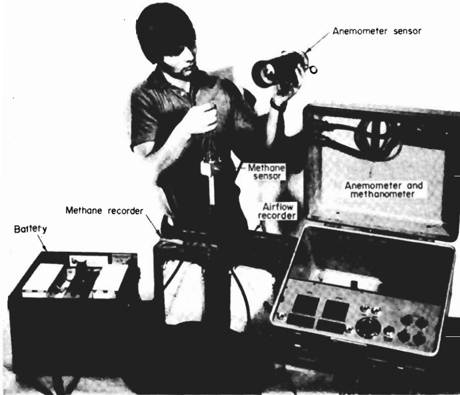
FIGURE 6. - Combined anemometer-methanometer instrument package.
