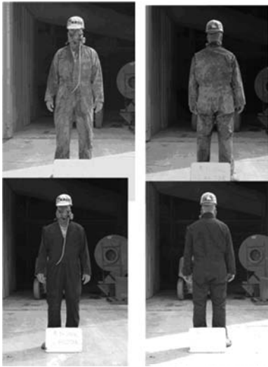
Figure 5. Before cleaning (top) and after cleaning (bottom) using clothes cleaning system.
