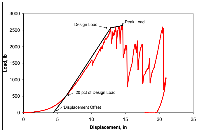
Figure 3. Load displacement curve for a test on a welded wire screen showing key parameters used to evaluate the screen performance.
