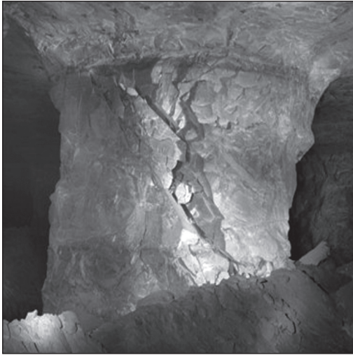
Figure 1. Partially benched pillar that failed along two angular discontinuities. Width-to-height ratio is 0.58 based on full benching height and average pillar stress is about 4% of the UCS.
